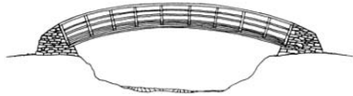
A graceful arched bridge constructed from laminated timber (Glu lam) and with ends finished neatly by stone walling.
