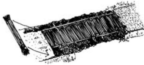
Path construction using fascines or faggots of brushwood pegged into place and covered with crushed stone. This is an old, well-tried method.
