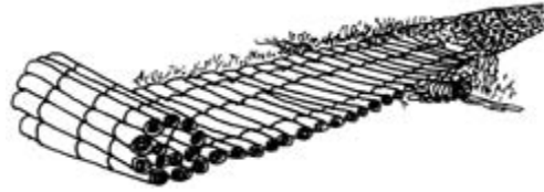
Rafting construction using lengths of timber wired together into a continuous mat. This is laid straight onto the surface once any basic preparation has been carried out. Path surfacing is laid over this, covering the timber to keep out the air.
