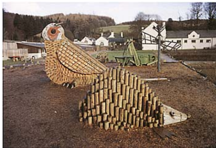
24 Part of a play area at Grizedale Forest, Cumbria, England. Here sculptors have created play equipment based on different kinds of wild animal. The pheasant is a slide. Note the extensive use of bark as a safety surface, retained by a log edge. This is an ideal surface to use in outdoor areas.
