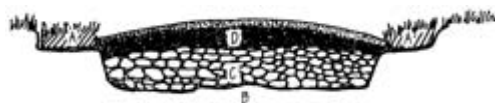
A typical section diagram to show path construction on firm, freely drained ground: (a) Turves are stripped and retained to be used to tidy the edge of the path after construction. (b) The path route is excavated down to firm subsoil, and large
