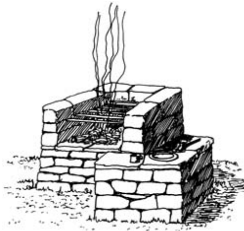
This design incorporates a fixed grill and a lower table on which to place plates, utensils etc.
