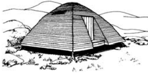
A specially designed beehive-shaped mountain shelter made of a curved timber pole framework covered and floored with sawn timber. Designed and built by Charles Gulland for Scottish Natural Heritage.
