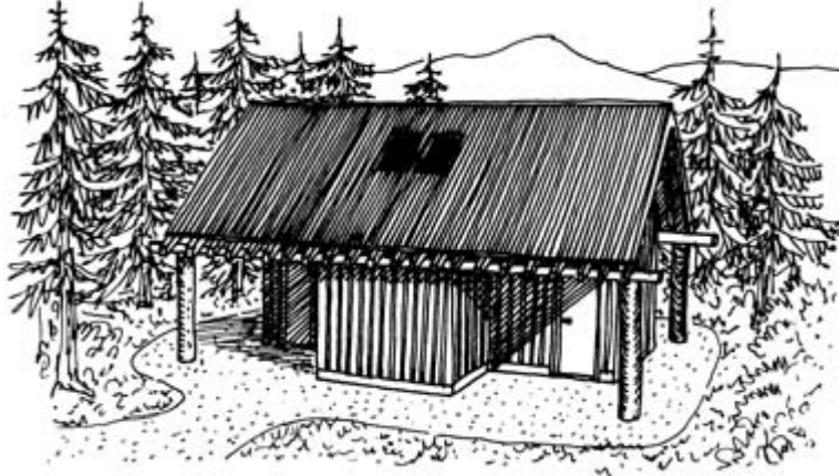
A toilet building designed for a forest landscape. Coarse textures of cladding and roof, exposed beam ends and the use of large dimension timbers work rather
