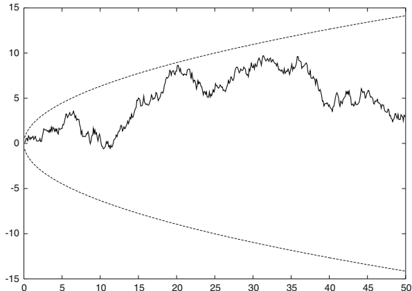
Fig. 1 Simulation of a Brownian motion with the 95 %-confidence interval curves f_{\pm}(t) = \pm 2\sqrt{t}
