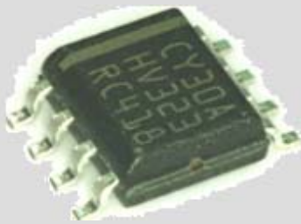
Sensor interface for an inductive engine wheel speed single rotation sensor
