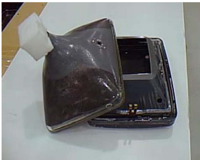
Fig. 9. CRT components separated by saw cut.
