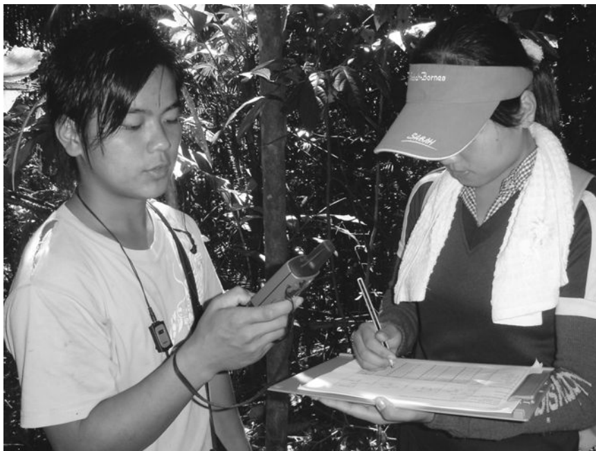
Figure 10.2 Buayan, Malaysia, research assistants collect GPS points in the process of ground truthing locations on their community map.
