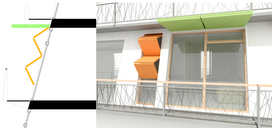
Figure 4.2.5 Illustration - Shading device - Typical summer sunny day option
