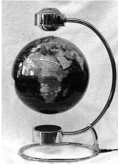
Fig. 14.21 Floating globe using magnetic suspension with feedback.
