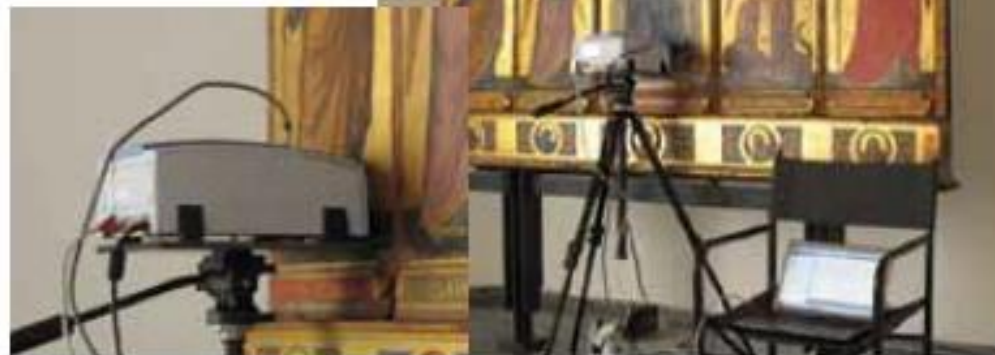
Figure 6: Polittico di Giotto with a tripod mounted ALPHA-R and a laptop PC.
