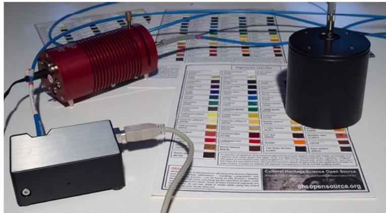
Figure 1. Miniaturised FORS system (from left to right): halogen lamp, USB4000 spectrometer and integrating sphere.
