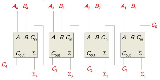
The output carry  $(C_4)$  is not ready until it propagates through all of the full adders. This is called *ripple carry*, delaying the addition process.
