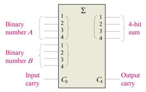
The 74LS283 is an example. It features *look-ahead carry*, which adds logic to minimize the output carry delay. For the 74LS283, the maximum delay to the output carry is 17 ns.
