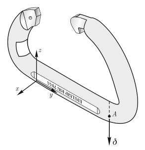
Fig. 1.11. Location of point A for which the vertical displacement is sought
