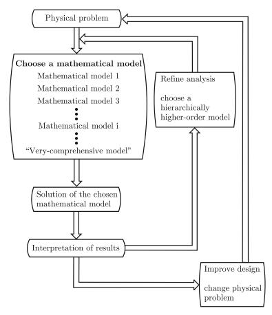
Fig. 1.13. The process of engineering design
