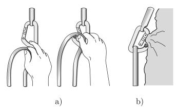
Fig. 1.3. Schematic representation of the carabiner usage and of a situation that makes it to work open
