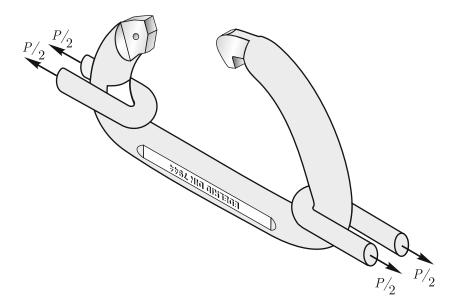
Fig. 1.9. Model of the carabiner with ropes included
