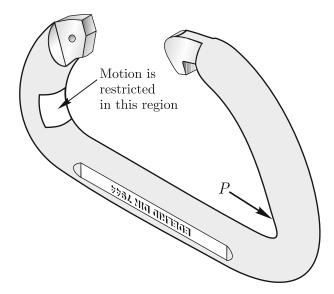
Fig. 1.4. Model representation of loading and boundary conditions
