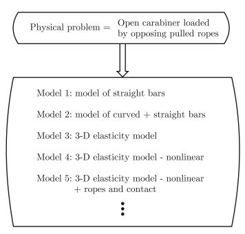
Fig. 1.10. Sequence of hierarchical models for the carabiner
