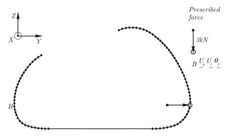
Fig. 1.6. Straight bar model in Y-Z plane. The material of the carabiner is aluminum with E = 70 GPa,  $\nu = 0.33$
