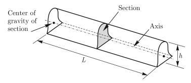
Fig. 1.5. A typical bar obtained by extruding a plane section through a straight line, normal to the plane of the section. The line, or axis, passes through the plane's center of gravity
