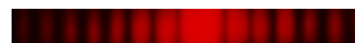
v / Single-slit diffraction of red light. Note the double width of the central maximum.
