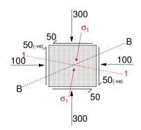
Plane BB is inclined at 20° to the horizontal
