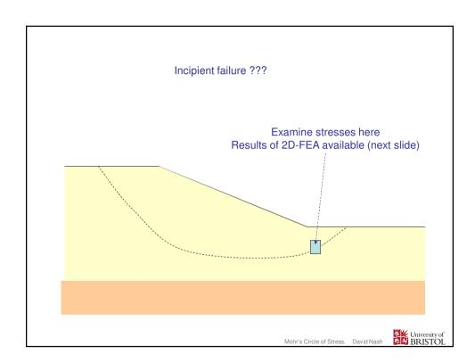
A plane strain finite element analysis is made in order to predict the stress conditions at various critical locations of a proposed excavation. The results show that the total normal and shear stresses (in kPa) at one such critical location, at the end of construction, will be as shown below. The pore pressure is 60 kPa.
