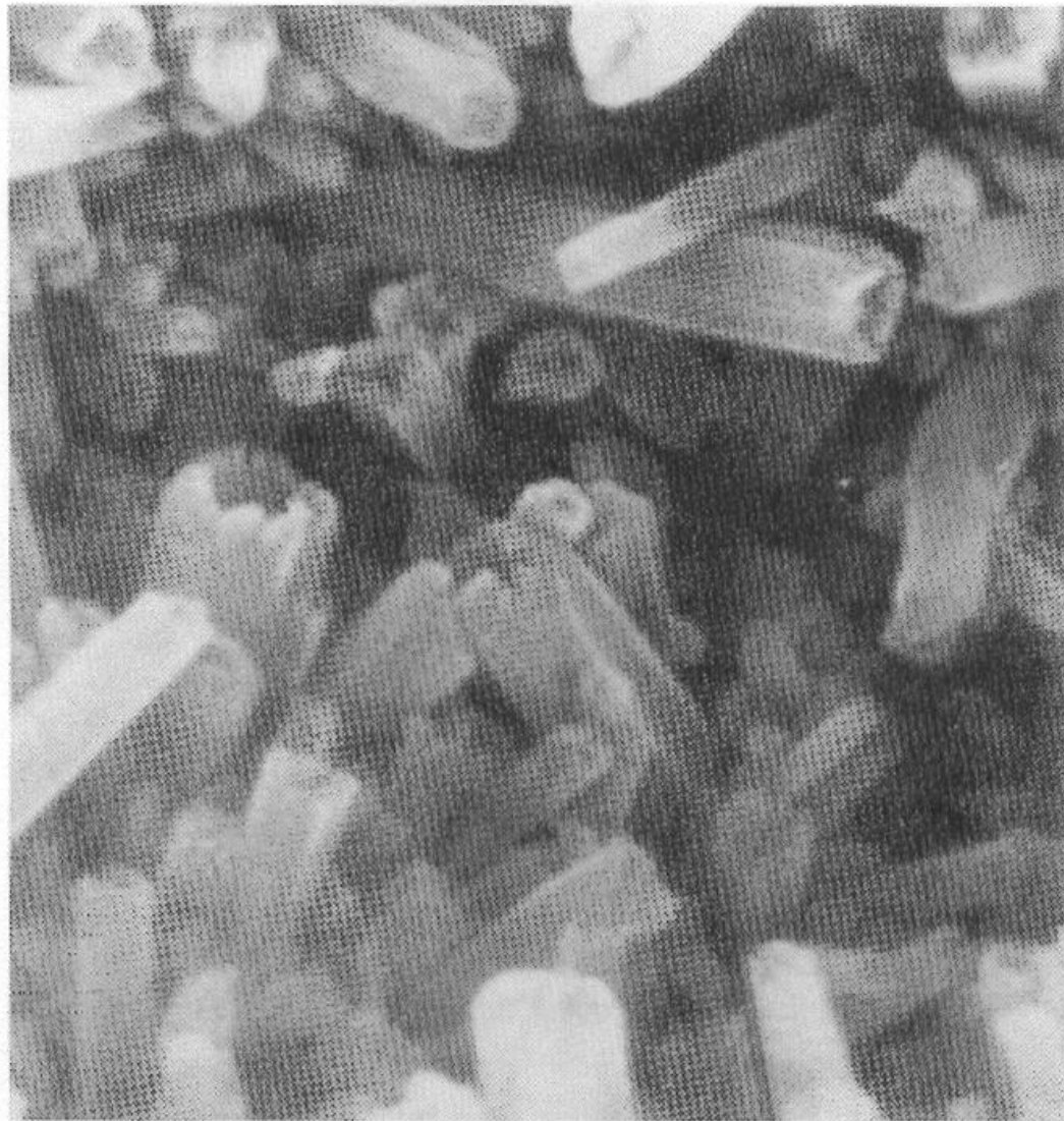
Figure 3.14 Electron photomicrograph of halloysite from Bedford, Indiana. Picture width is 2\ \mu\text{m} (Tovey, 1971).
