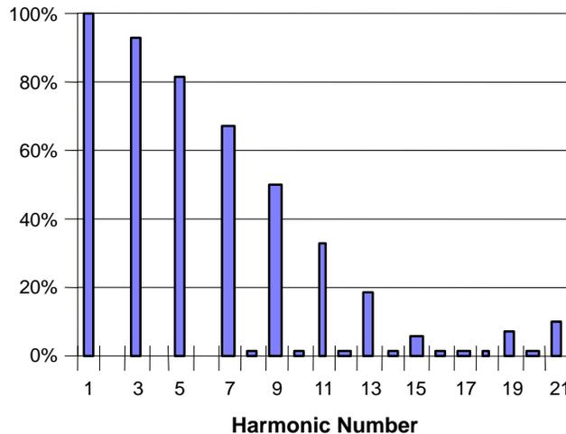
**Figure 1–2. Harmonic Content of the Current Waveform in Figure 1–1**
