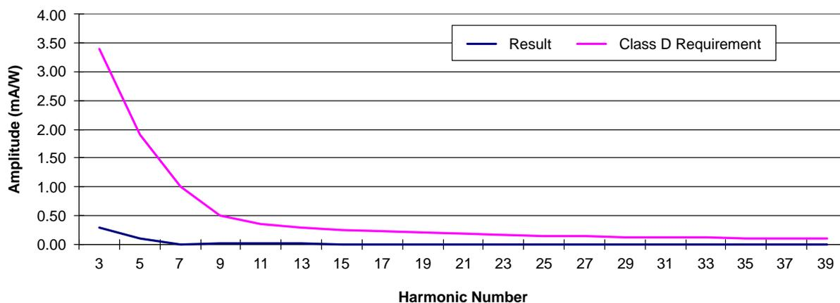
Figure 4–5. Harmonic Spectrum of 270 W FCCrM Converter at Full Load
