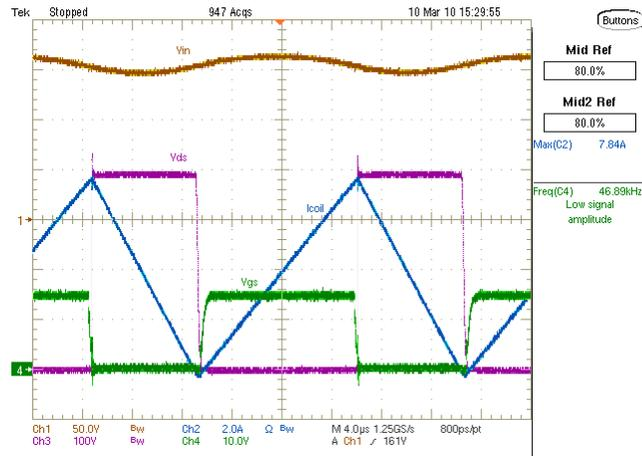
**Figure 4–8. Switching Waveforms at Full Load, 115 Vac Input**
