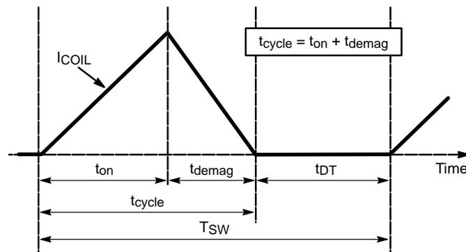
Figure 1-13. DCM Operating Waveforms
