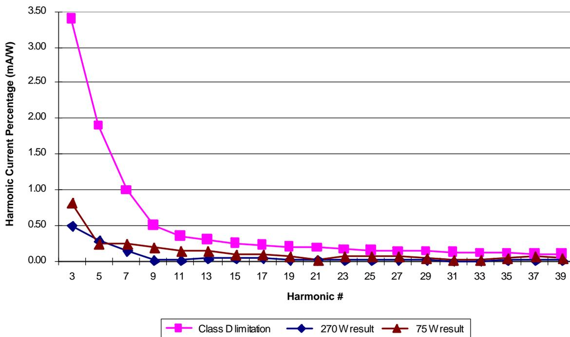
Figure 3-4. Harmonic Content of NCP1607 Based PFC Converter at Full Load and 75 W
