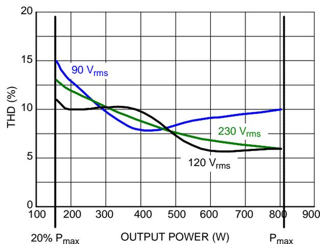
Figure 8–14. Total Harmonic Distortion Over the Load Range
