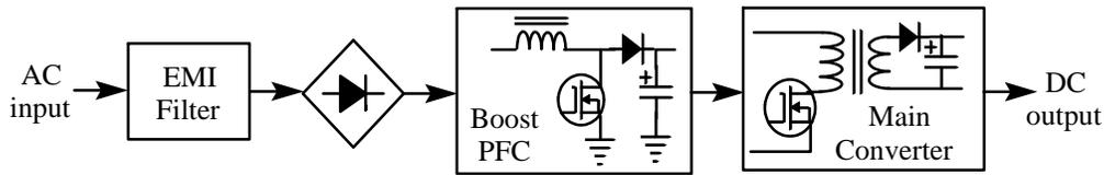
Figure 9–1. Conventional Two-Stage Conversion
