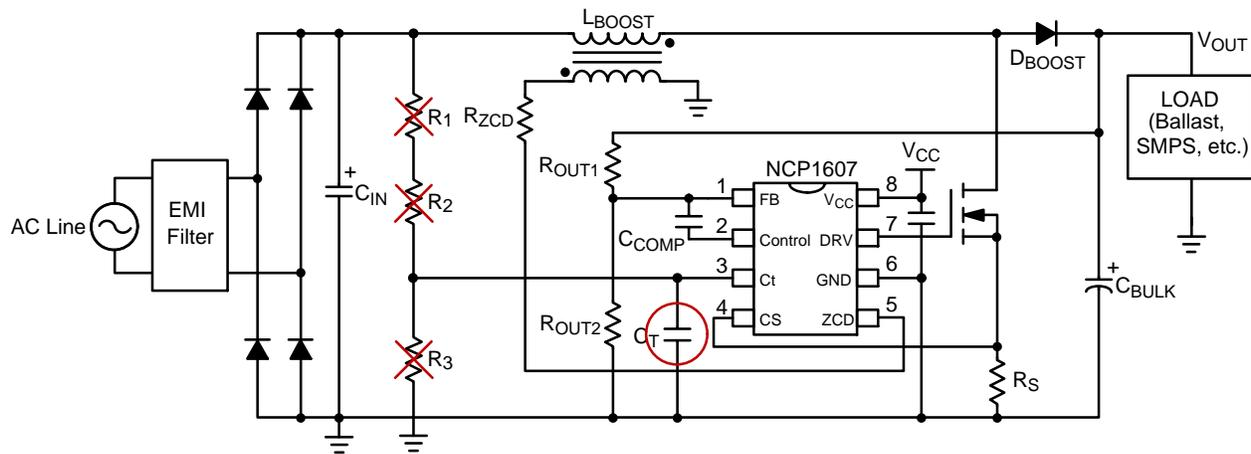
Figure 3–2. Converting from Current-Mode Control to the NCP1607
