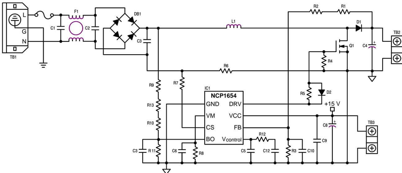
Figure 6–3. Circuit Schematic of the CCM PFC Circuit Based on NCP1654
