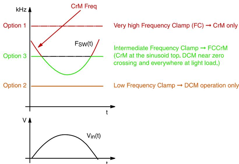
Figure 1–15. PFC Mode Selection Through Frequency Clamping
