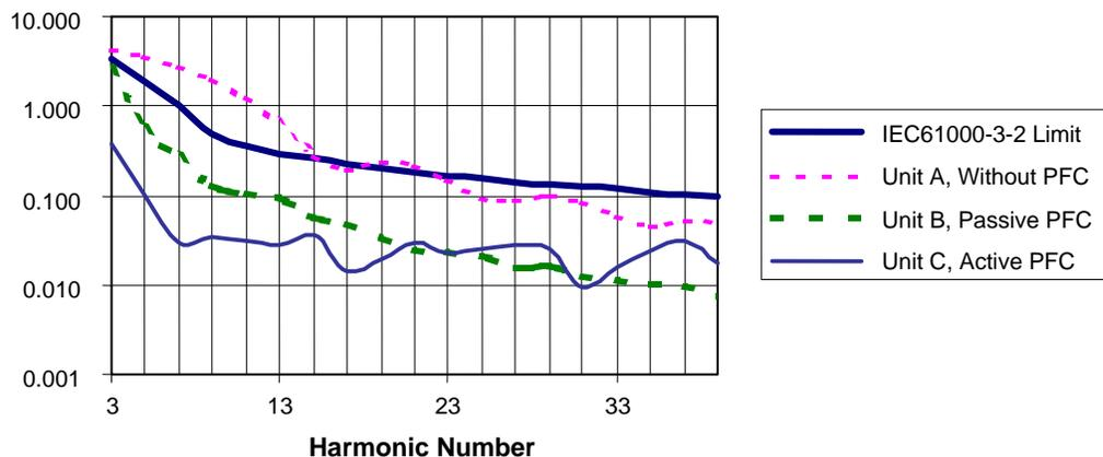
Figure 1-6. Input Harmonics of Three PC Power Supplies Relative to IEC61000-3-2 Limits
