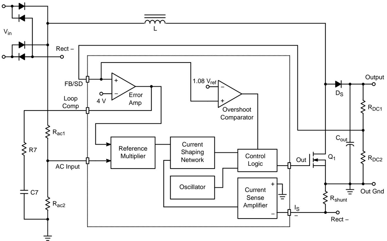
Figure 1-19. Simplified Block Diagram of the NCP1650 PFC Controller
