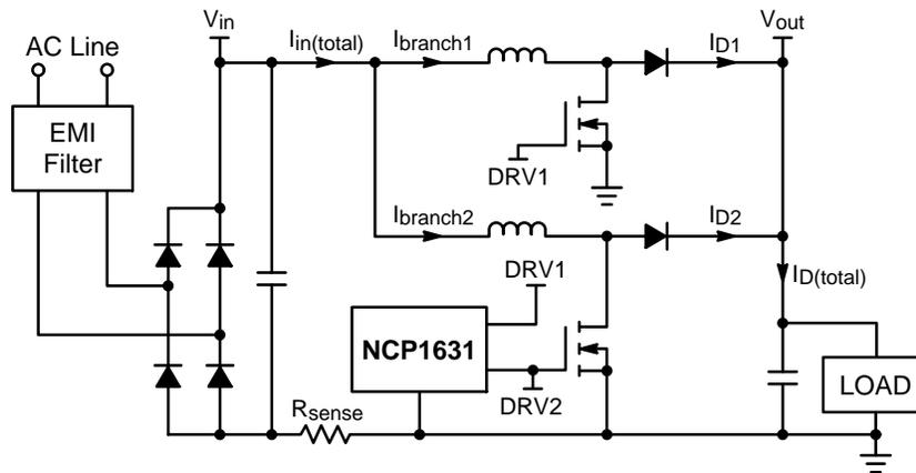
Figure 7-2. Simplified Schematic of an Interleaved PFC Stage
