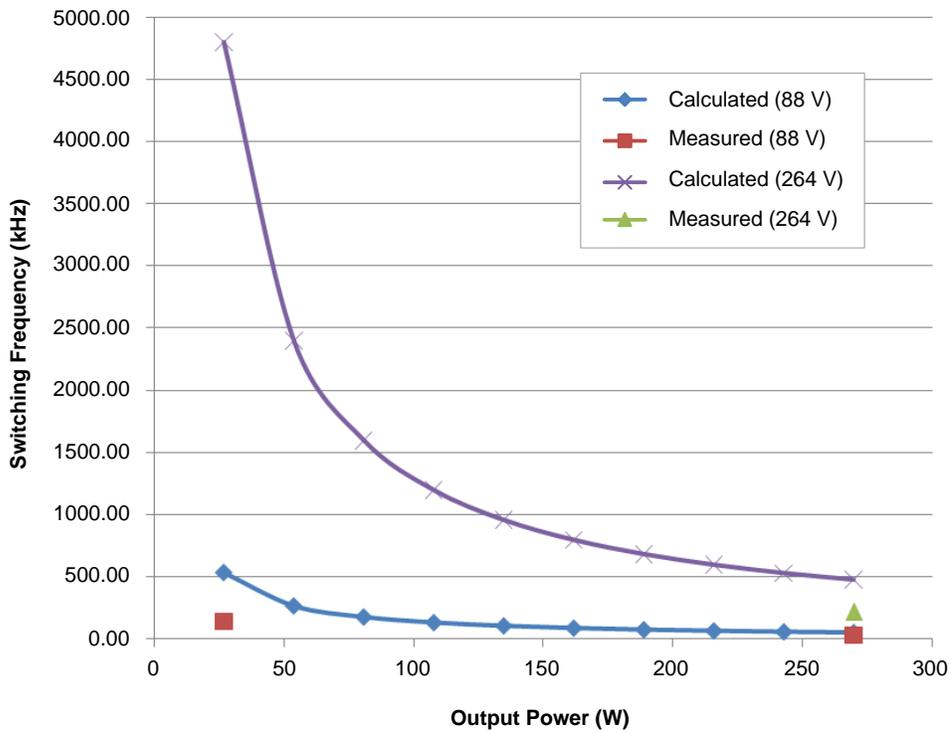
Figure 3-7. Frequency Variation at Zero Crossing in CrM PFC
