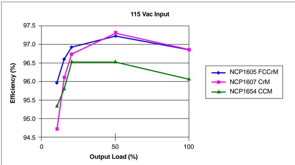
Figure 10-4. Efficiency Performance at 115 Vac
