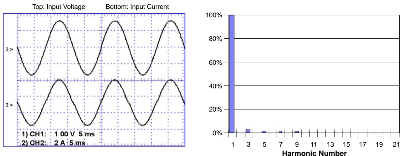
Figure 1–3. Input Characteristics of a Power Supply with Near-Perfect PFC
