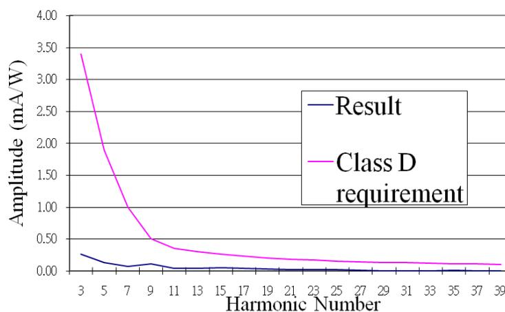
**Figure 6–4. Harmonic Spectrum of the 270 W CCM Converter**
