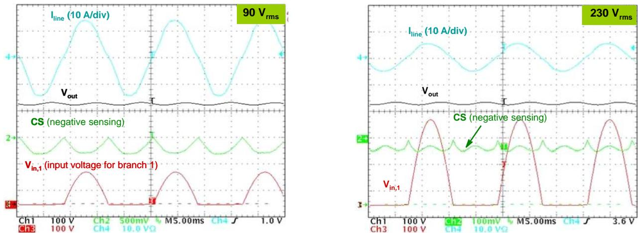
Figure 8–11. Typical Waveforms at Low Line (Left) and High Line (Right)
