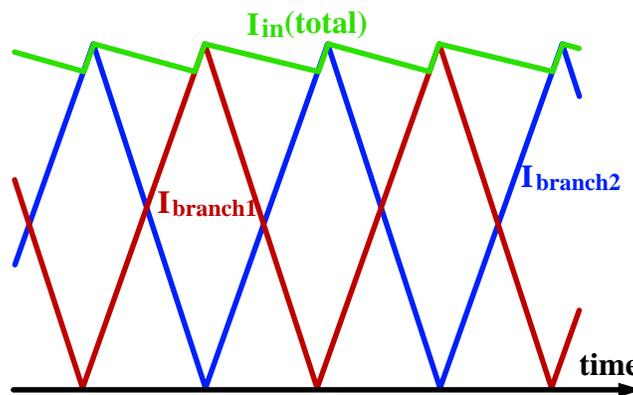
Figure 7-3. The Total Current Exhibits a Reduced Ripple
