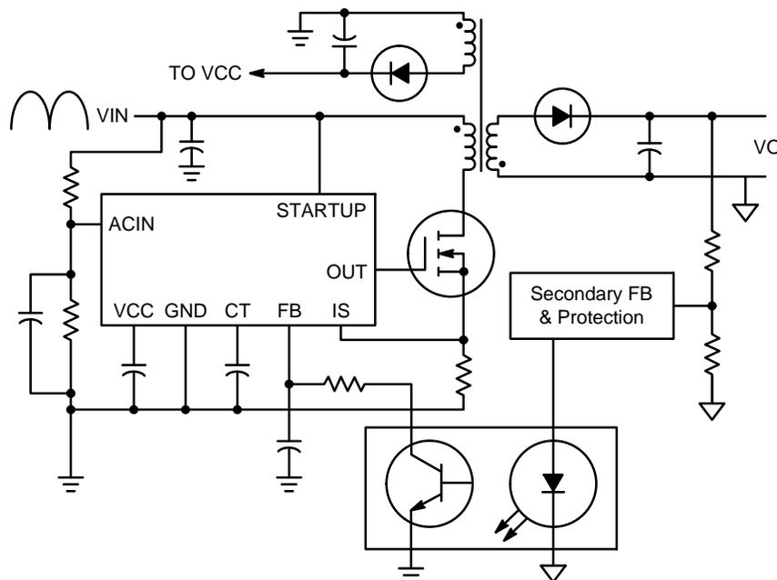
Figure 1-20. Single Stage PFC Using the NCP1652
