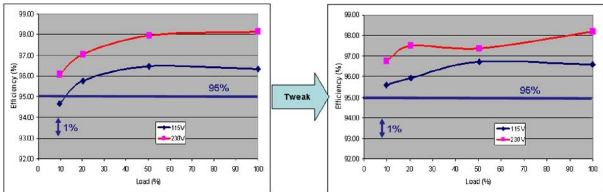
Figure 7-10. Tweaking the Frequency Fold-back Characteristic can Help Improve the Light-load Efficiency
