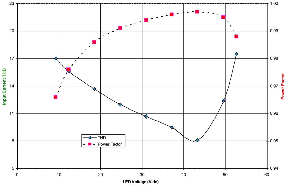
Figure 9-6. Power Factor and THD vs. Load (115 Vac Input)
