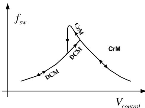
Figure 5–8. The System Enters and Leaves DCM in Accordance with the  $V_{control}$  Level
