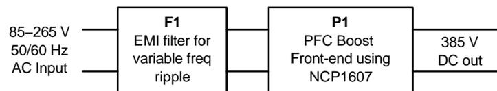
Figure 2–1. Critical Conduction Mode PFC
