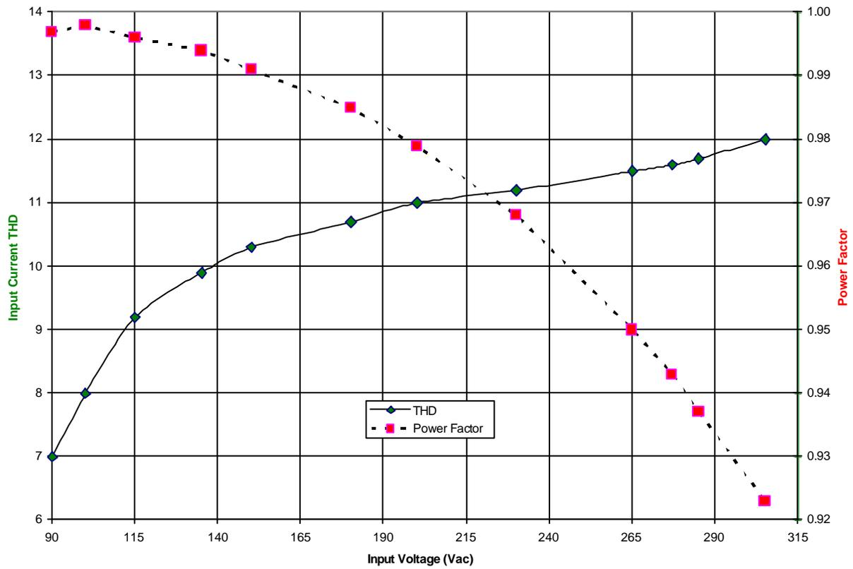
Figure 9-5. THD and Power Factor with 12 LED ( $V_f = 37$  Vdc) Load Over a Wide Input Range
