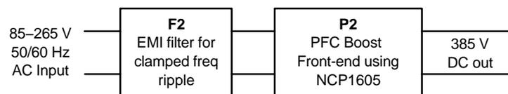
Figure 2–2. Frequency Clamped Critical Conduction Mode PFC
