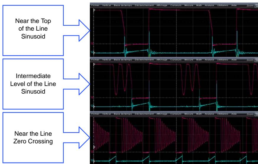
Figure 5-3. Operation @ 230 V, 160 W Near the Line Zero Crossing of the NCP1612 Evaluation Board. The MOSFET Drain-source Voltage is in Red, the Blue Trace Showing the MOSFET Current.
