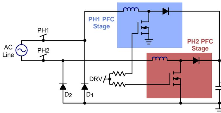
Figure 8–3. Two-Phase Architecture
