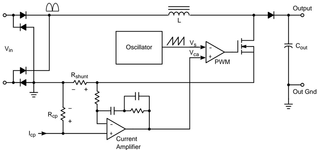
Figure 1–18. Diagram for Average Current Mode Control Circuit
