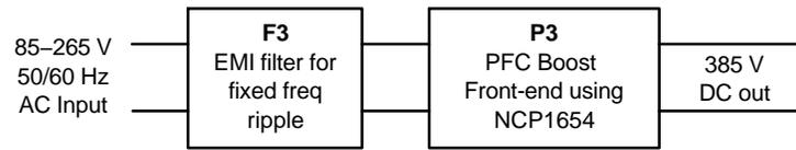
Figure 2–3. Continuous Conduction Mode PFC
