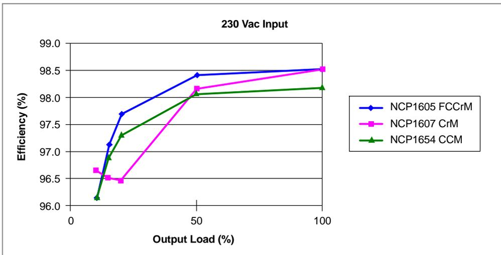
Figure 10-5. Efficiency Performance at 230 Vac
