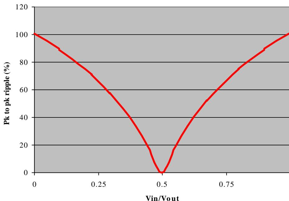
Figure 7–4. Peak-to-Peak Ripple of the Input Current as a Function of the Line Magnitude
