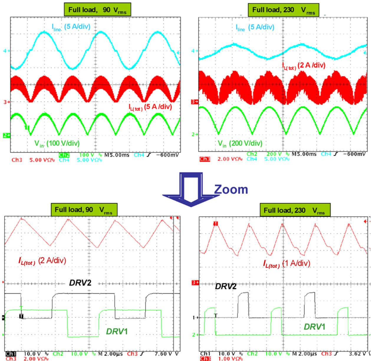
Figure 7–8. Typical Waveforms at Full Load
