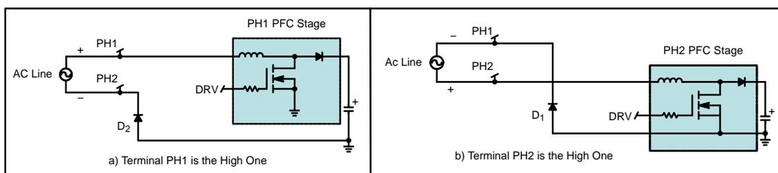
Figure 8–4. Equivalent Schematic for the Two Half-Waves
