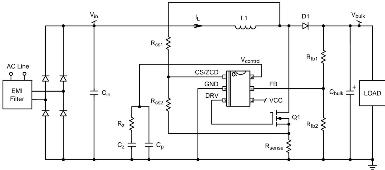
**Figure 5-7. Generic Application Schematic for the NCP1602 6-pin Controller that Embeds the VSFF Technique**
