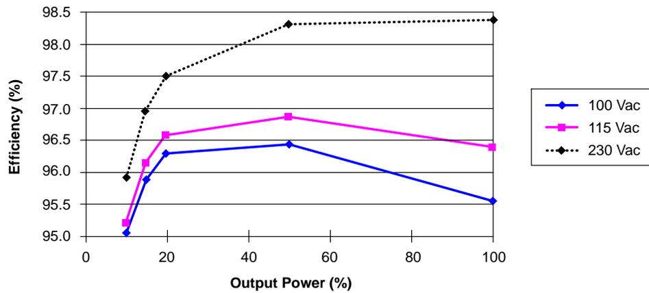
Figure 4-9. Efficiency Plot for FCCrM PFC
