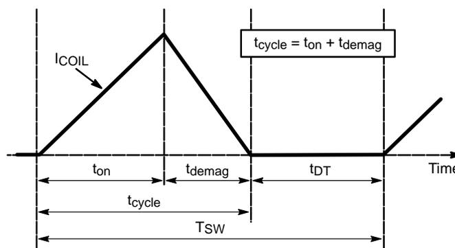
Figure 4–1. States of Operation in Discontinuous Conduction Mode PFC
