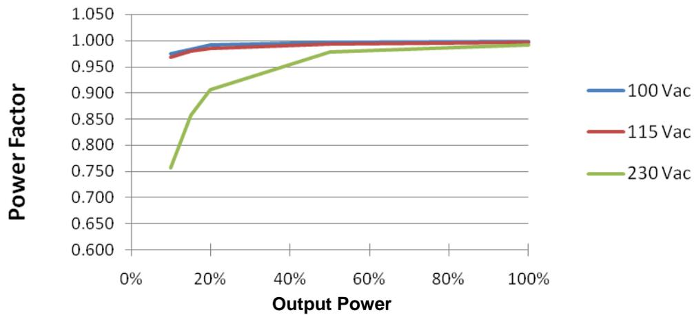
Figure 6–6. Power Factor Performance of the 270 W CCM Design
