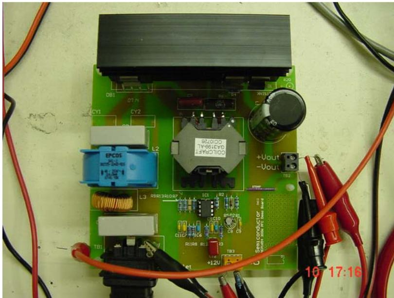
Figure 10–1. Picture of NCP1654 Demo Board Used for Comparisons
