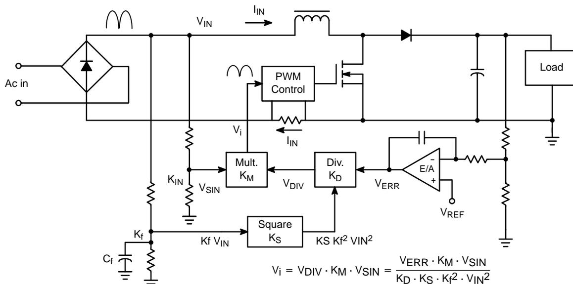
Figure 1–17. Block Diagram of the Classic PFC Circuit
