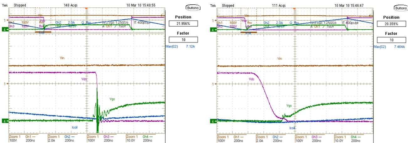
Figure 4–7. Turn-On Waveforms with (Left) No ZCD Delay and (Right) Optimized ZCD Delay
