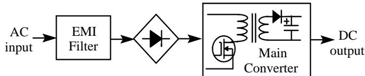
Figure 9–2. Single Stage Conversion with NCP1652
