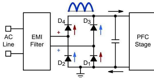
**Figure 8–1. The Input Current Flows Through Two Diodes**
