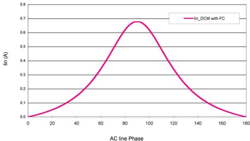
Figure 1–12. CrM Line Current Distortion Due to Frequency Clamping
