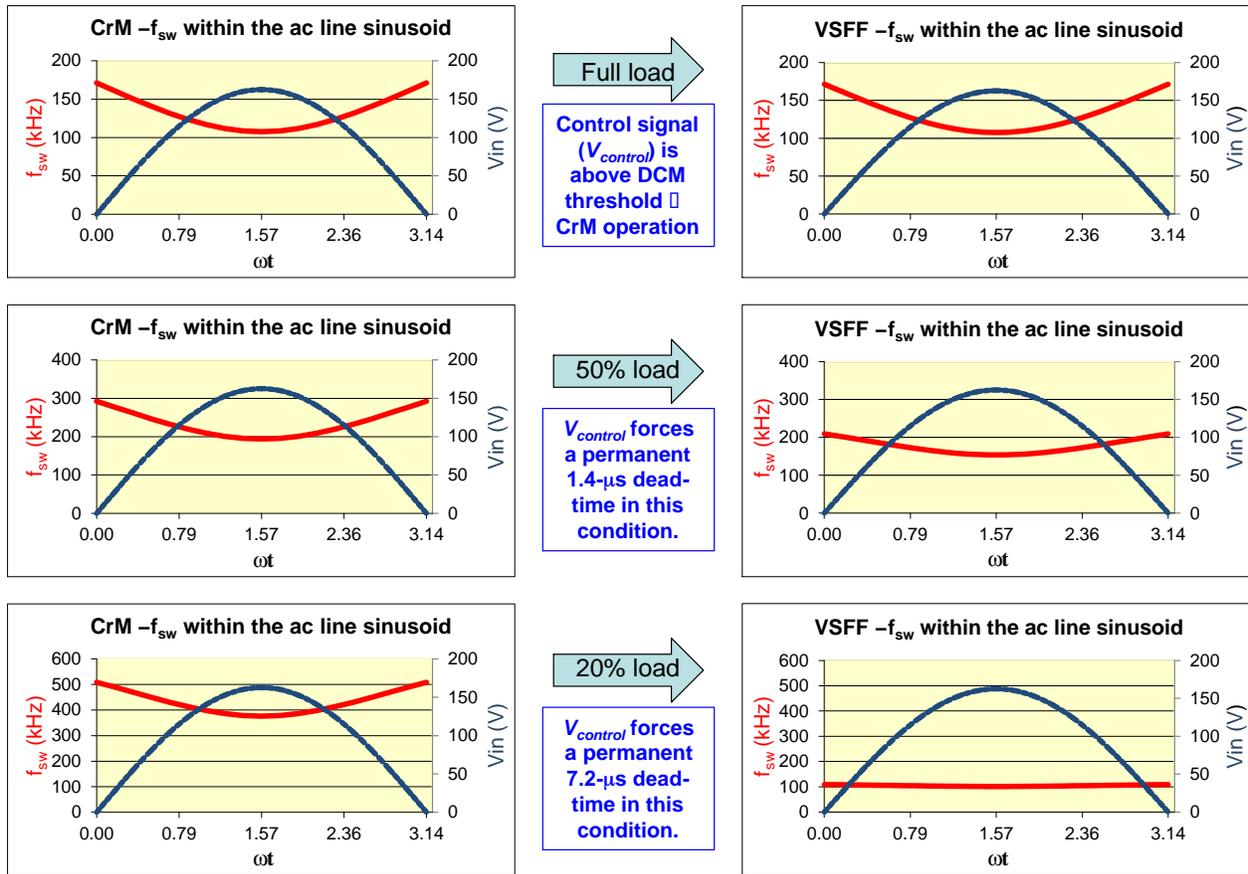
Figure 5-11. VSFF with Respect to CrM at Three Different Load Levels
