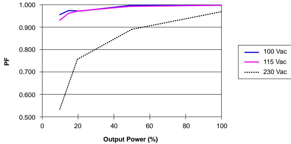
Figure 3-9. Power Factor Performance Over Line and Load
