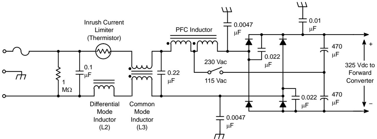
Figure 1–7. Passive PFC in a 250 W PC Power Supply
