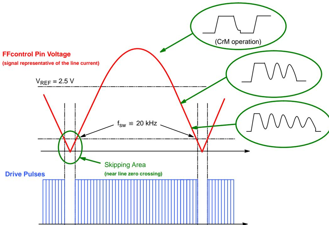
Figure 5-1. Current-Controlled Frequency Fold-back
