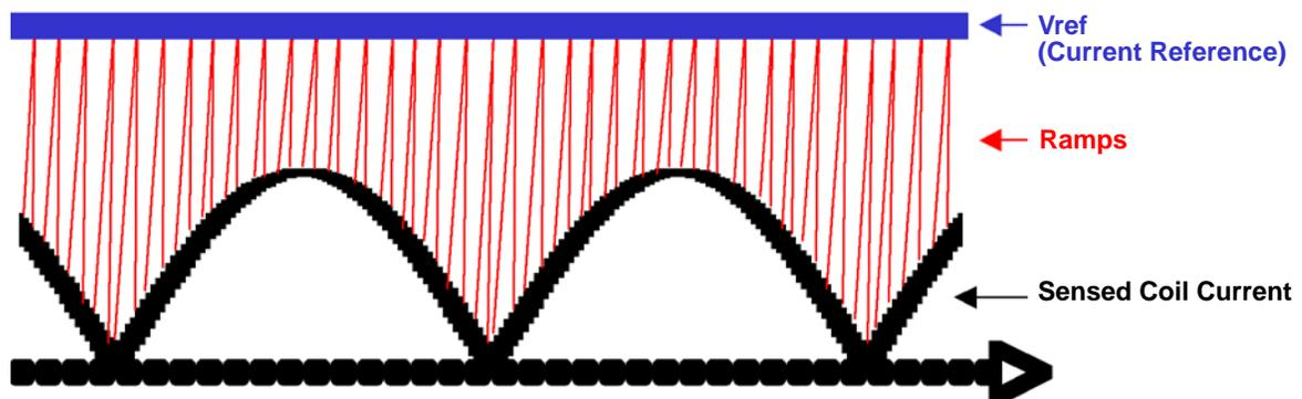
Figure 1–21. Predictive CCM Control Waveforms
