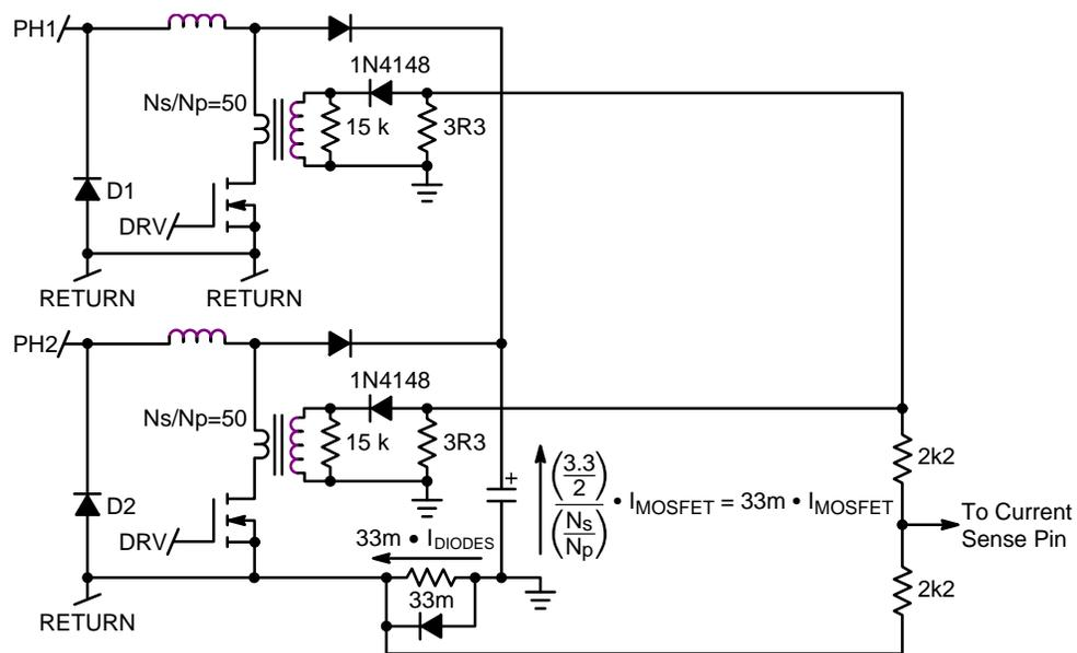
Figure 8–8. Details of the Current Sense Circuits
