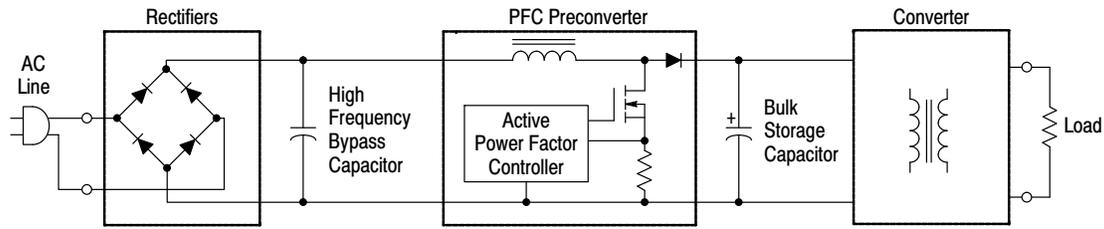
Figure 1-4. PFC Preconverter Stage
