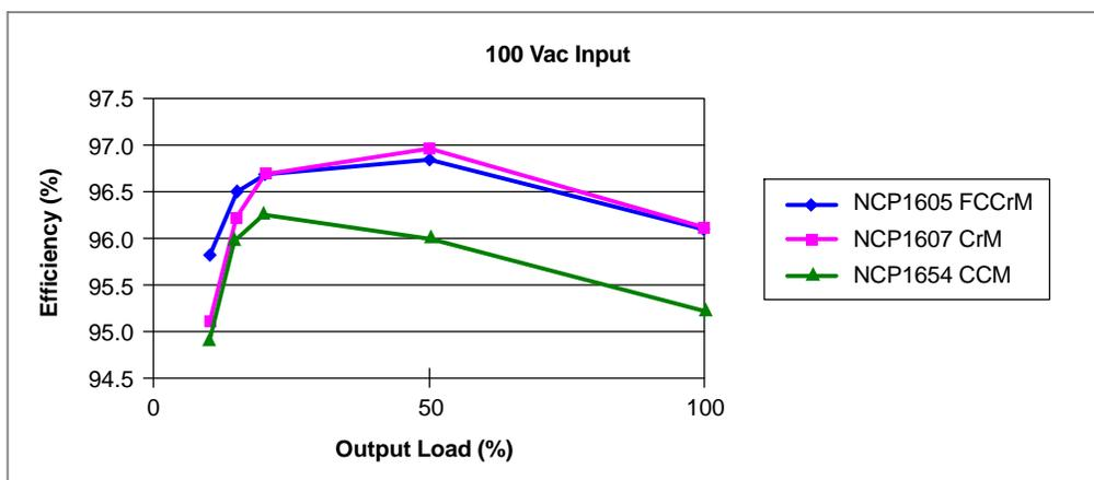
Figure 10–3. Efficiency Performance at 100 Vac
