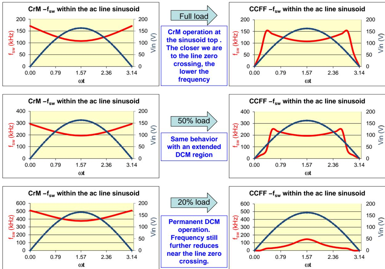
Figure 5–10. CCFF with Respect to CrM at Three Different Load Levels
