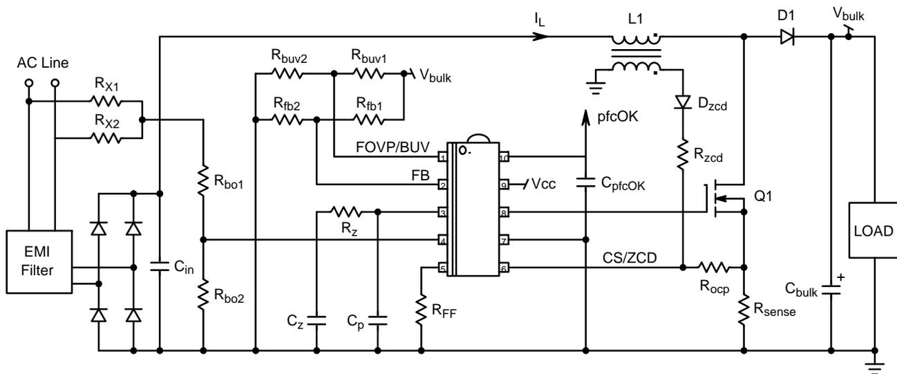
Figure 5–9. Generic Application Schematic
