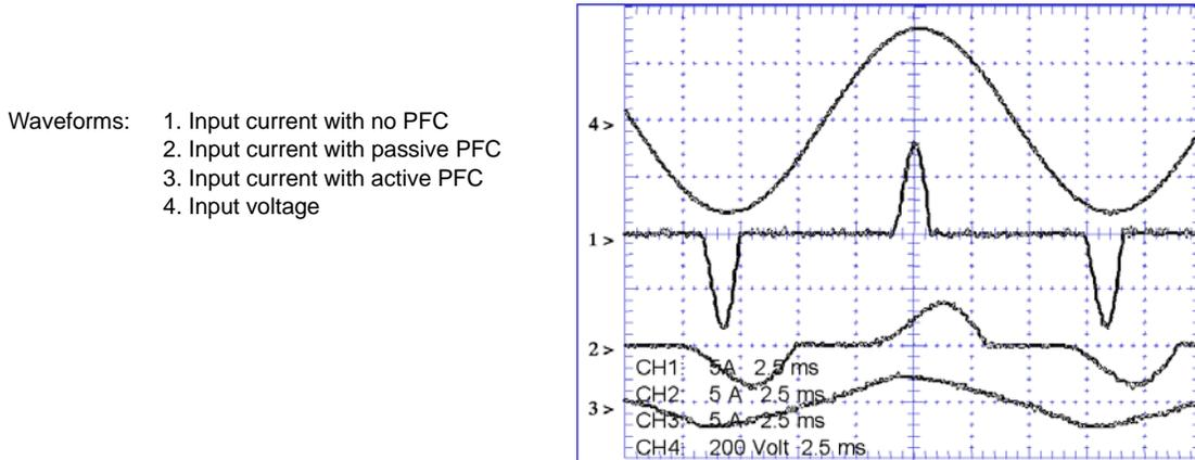
Figure 1-5. Input Characteristics of PC Power Supplies with Different PFC Types (None, Passive, and Active)
