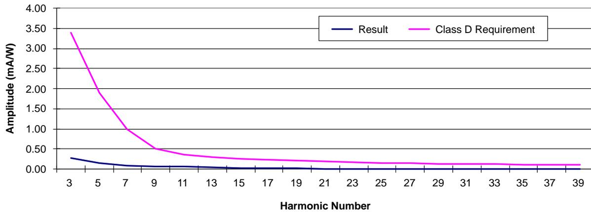
Figure 4–6. Harmonic Spectrum of 270 W FCCrM Converter at 75 W Load
