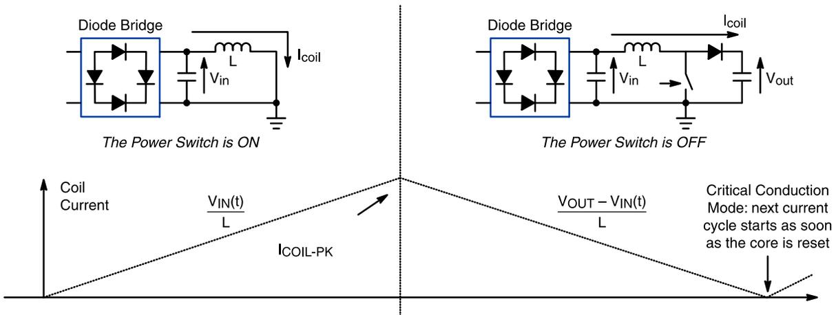
Figure 3–1. States of Operation in Critical Mode Conduction PFC
