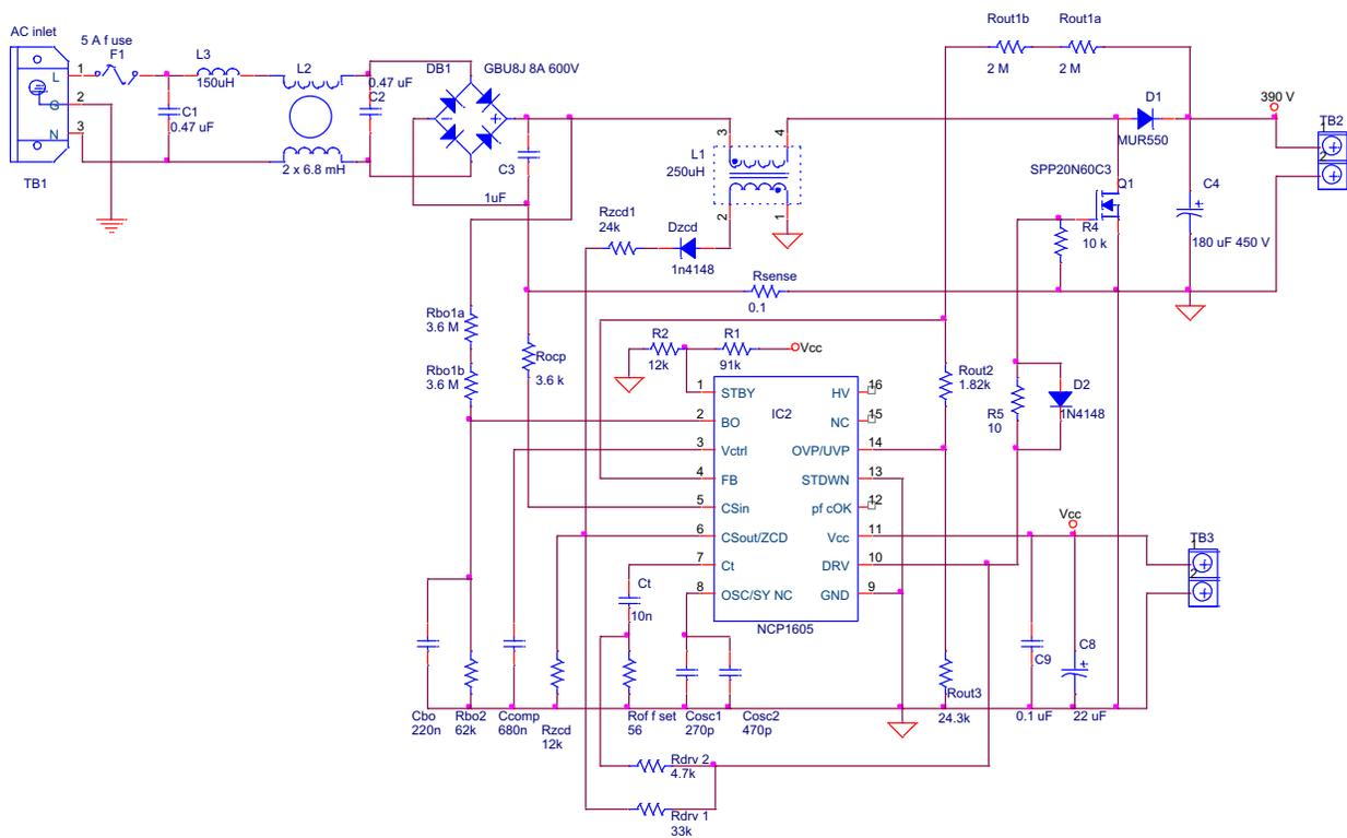
**Figure 4–4. Circuit Schematic of NCP1605 Based PFC Converter**
