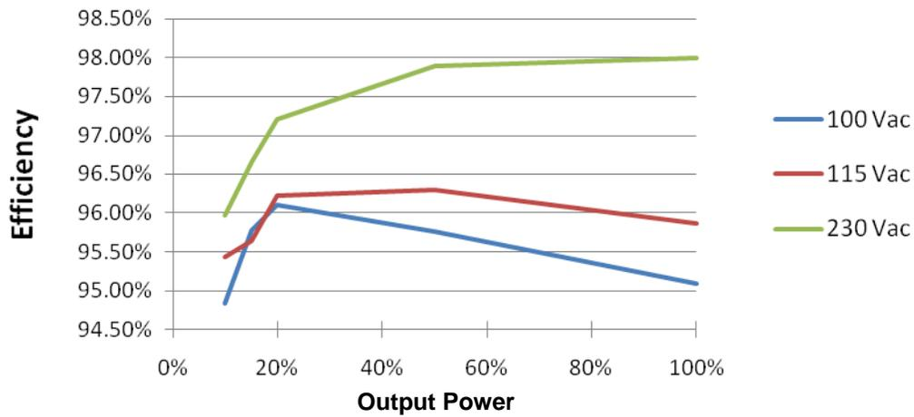
Figure 6–5. Efficiency Performance of the 270 W CCM Design
