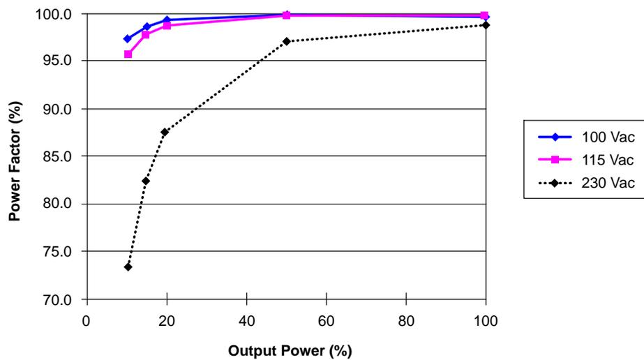
Figure 4-10. Power Factor Plot for FCCrM PFC
