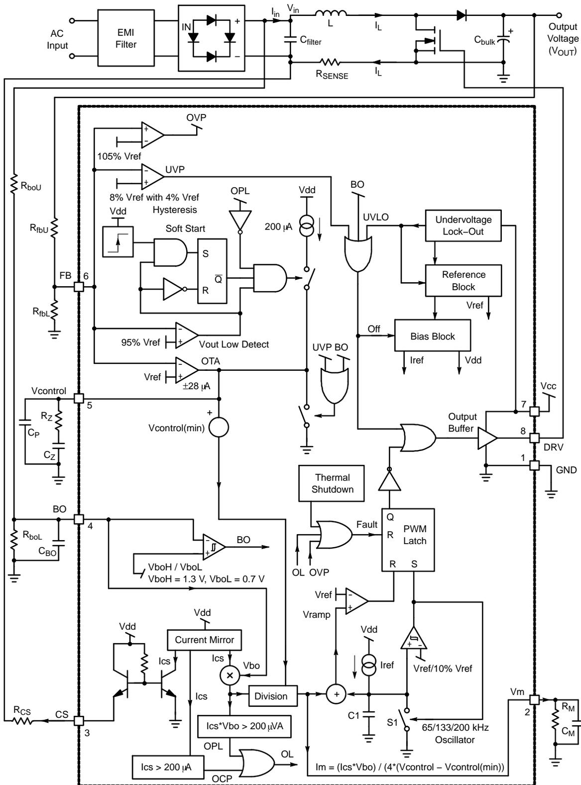
Figure 6-1. NCP1654 Block Diagram
