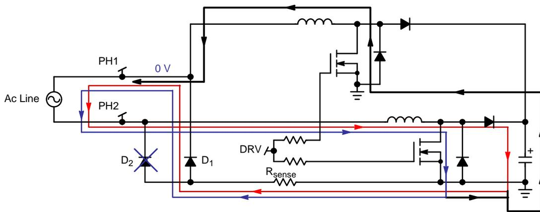
Figure 8-5. Operation for the "PH2" Half-Wave
