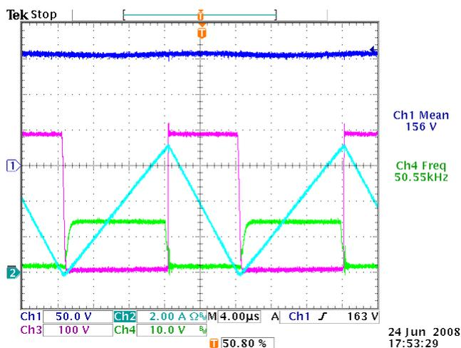
Figure 3–5. Operating Waveforms at Full Load, 115 Vac
