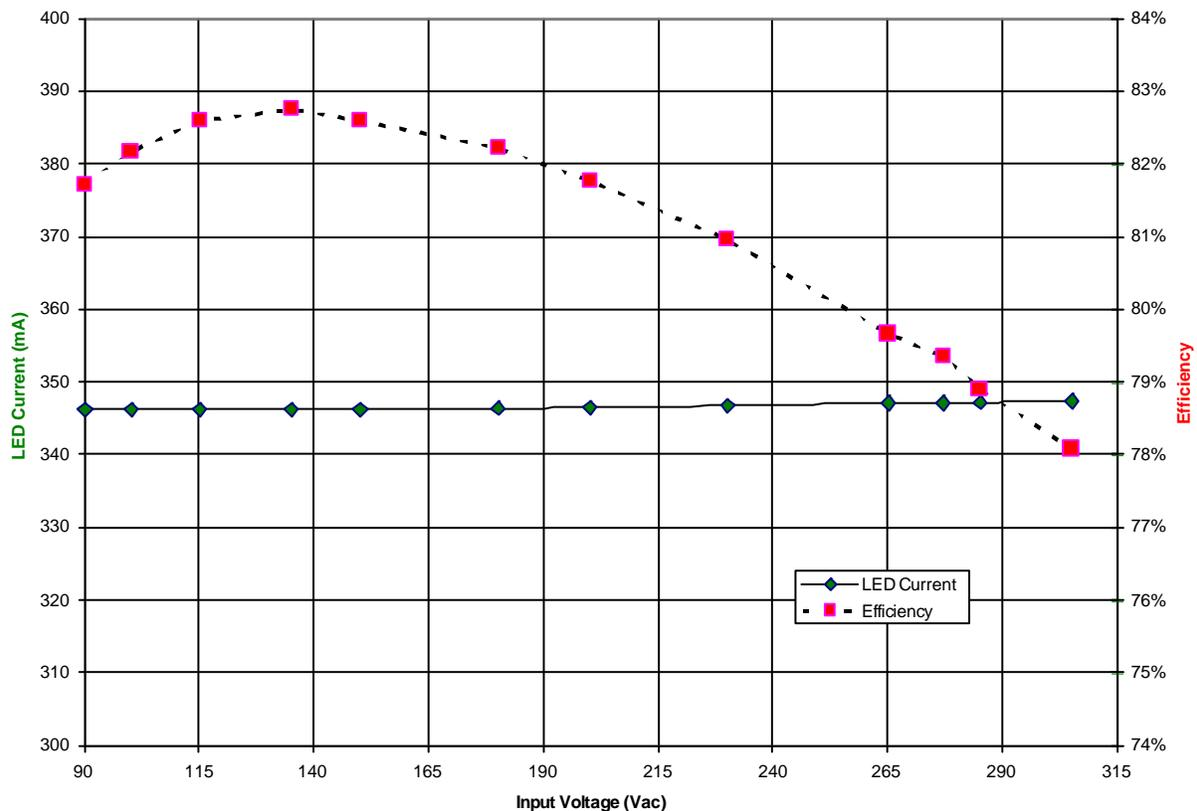
**Figure 9–4. Line Regulation and Efficiency Driving 12 LED Load ( $V_f = 37$  Vdc)**
