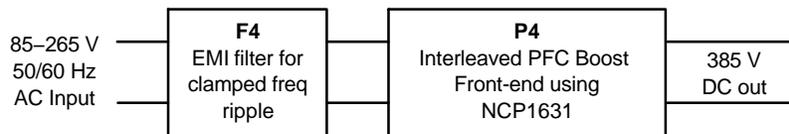
Figure 2–4. Interleaved PFC
