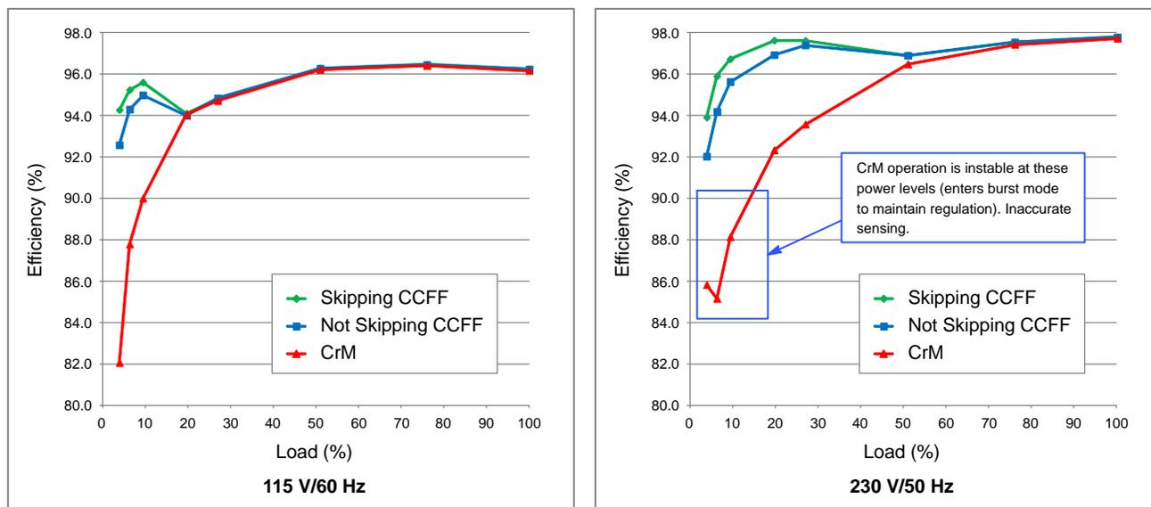
**Figure 5–5. Efficiency Over the Load Range at Low- and High-line Conditions**
