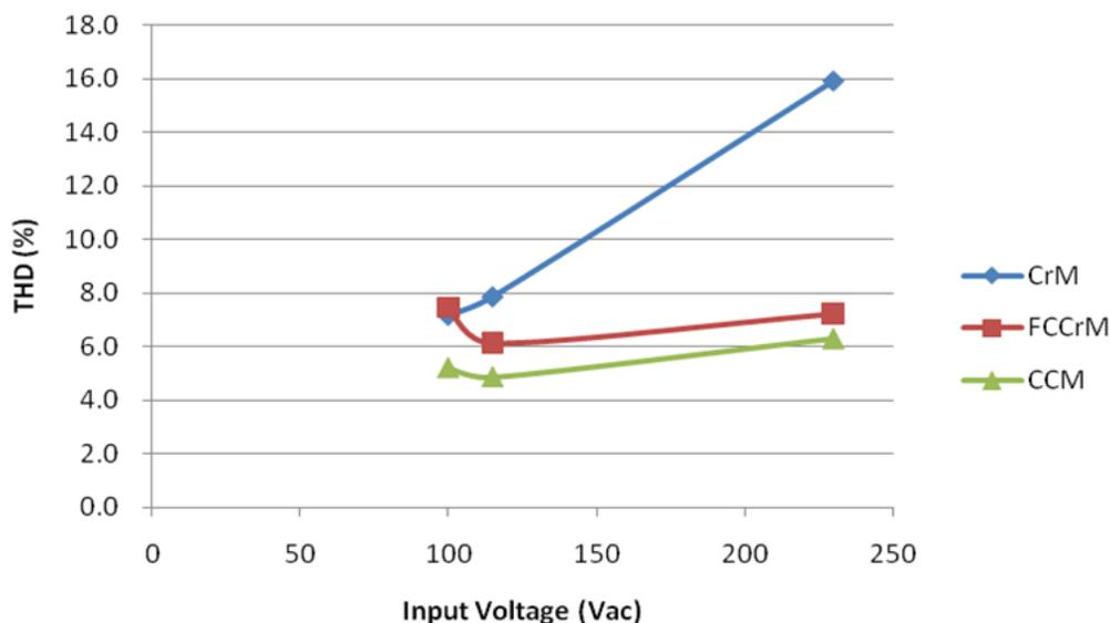
Figure 10-6. Total Harmonic Distortion Comparison
