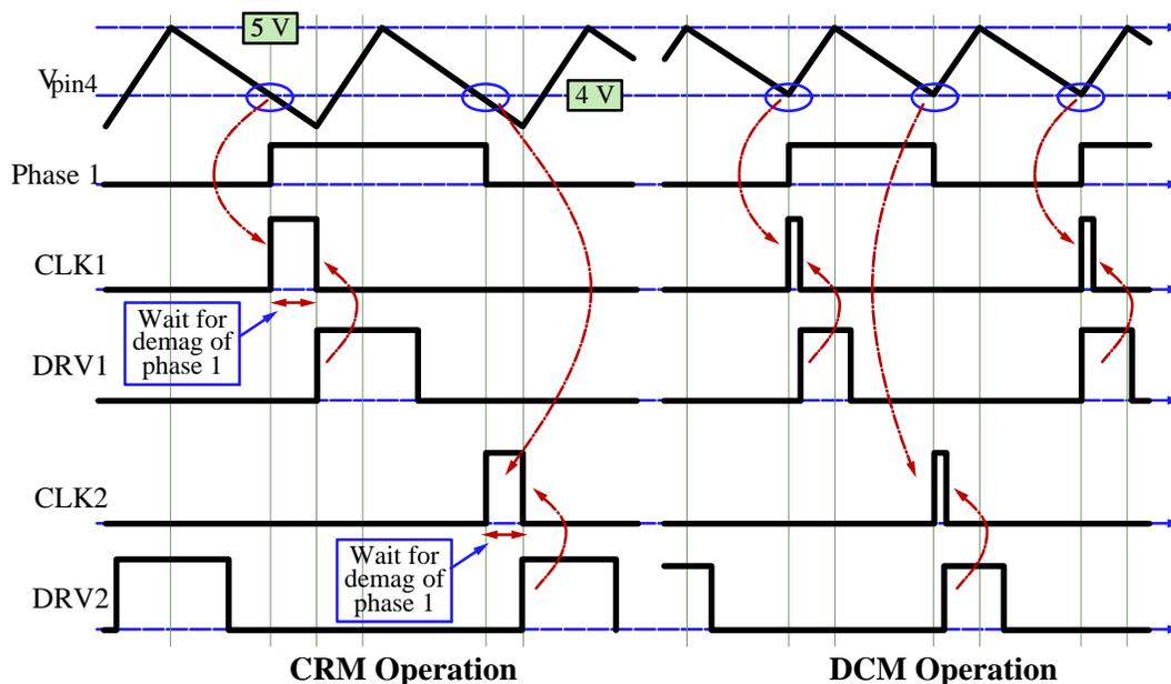
Figure 7–1. Interleaved Clock Generation
