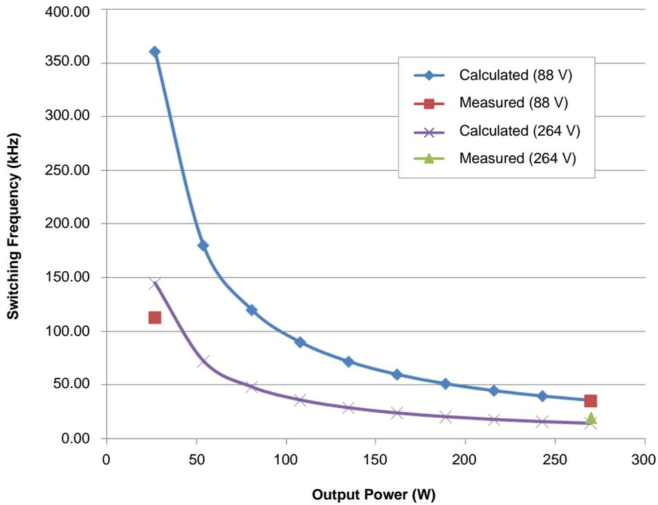
Figure 3-6. Frequency Variation at the Peak of the Sinusoid in CrM PFC
