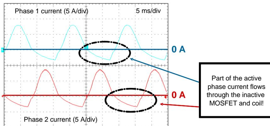
Figure 8-6. Part of the Current Flows through the Supposedly Inactive MOSFET and Coil
