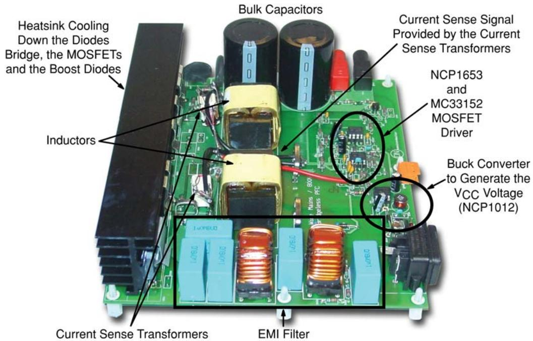
**Figure 8–9. Photograph of the Evaluation Board**
