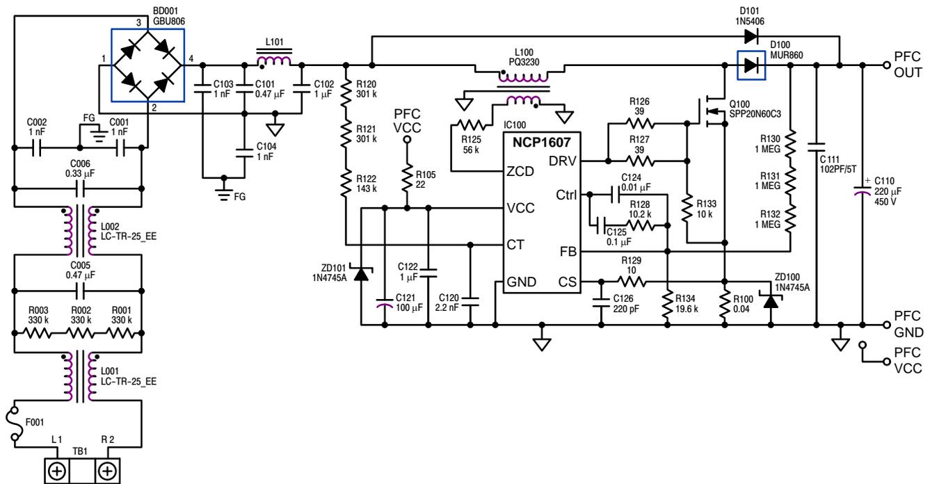
Figure 3–3. Schematic of NCP1607 Based PFC Converter
