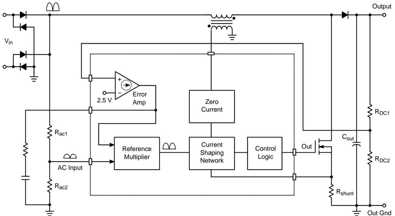
Figure 1-8. Basic Schematic for a Critical Conduction Mode Converter
