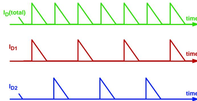
Figure 7-5. Reduction in the AC Content of the Refueling Current as a Result of Interleaving
