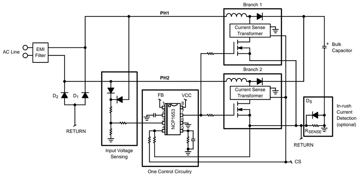
Figure 8–7. Simplified Application Schematic of Bridgeless Converter
