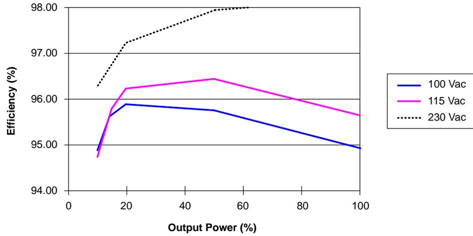
Figure 3-8. Efficiency Performance Over Line and Load
