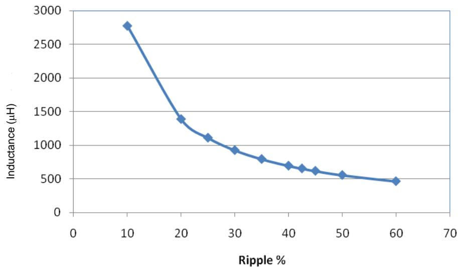
Figure 6-2. CCM Inductance Value as a Function of p-p Ripple
