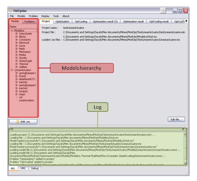
Figure 7.3: OMOptim window after having loaded model.
