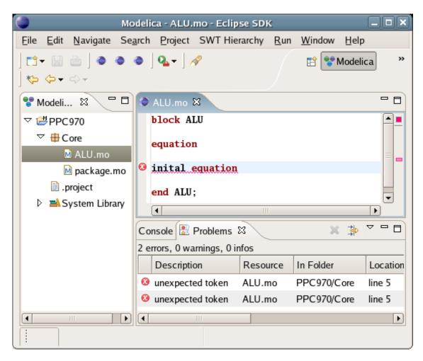
Figure 8.10: Syntax checking.
