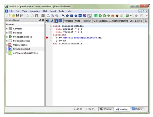
Figure 4.3: Adding breakpoint in Text View.
