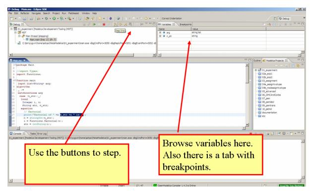
Figure 9.7: The debugging perspective.
