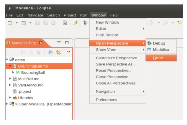
Figure 8.7: Eclipse – Switching to another perspective – e.g. the Java Perspective.
