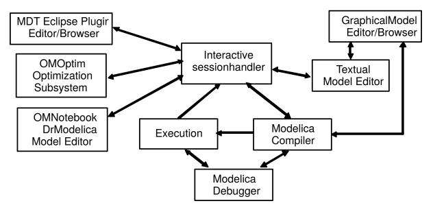
The OpenModelica environment consists of several interconnected subsystems, as depicted in Figure 1.1.
