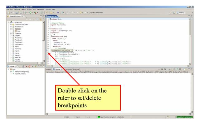
Figure 9.4: Setting/deleting breakpoints.
