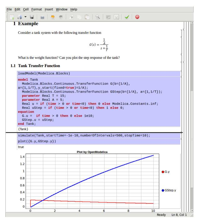
Figure 5.13: Step and pulse (weight function) response.
