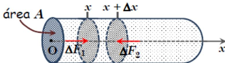
$$\begin{aligned} \Delta F &= \Delta F_1 + \Delta F_2 = P(x,t) A - P(x + \Delta x, t) A \\ &= -A \Delta x \left\{ \frac{P(x + \Delta x, t) - P(x, t)}{\Delta x} \right\} = -\Delta V \frac{\partial p}{\partial x}(x, t) \end{aligned}$$
