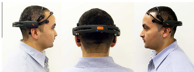
Fig. 3. Emotiv EPOC headset on a subject showing left, right, and back views.
