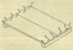
FIG. 53.—End of a box in course of making, to show the diagonal driving of the nails.
