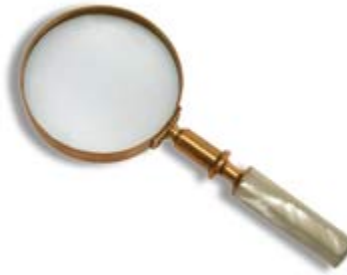
Fig. 4. The magnifying lens allows objects to be brought closer to the eye while still seeing them clearly. This produces an increase in their apparent size. F = focal length 250 mm = conventional distance of the near vision
