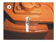
Fig. 5-3: Moving an axis to the pre-mastering position
