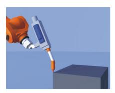
Fig. 5-24: Origin of the base coordinate system
