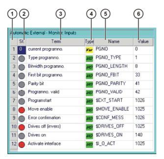
Fig. 4-27: Automatic External inputs (detail view)
