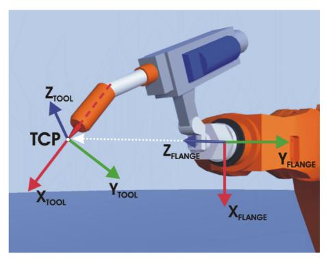
Fig. 5-8: TCP calibration principle
