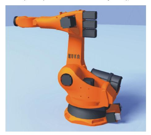
Fig. 5-2: Mastering position – approximate position
