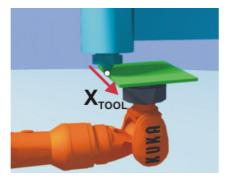
Fig. 5-20: Point on the positive X axis
