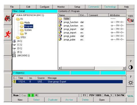
Fig. 2-2: KUKA.HMI user interface
