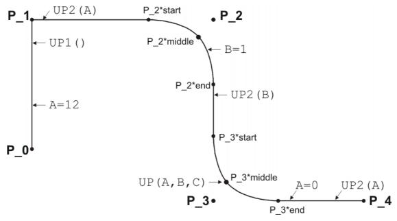
Fig. 10-12: Example of TRIGGER WHEN DISTANCE
