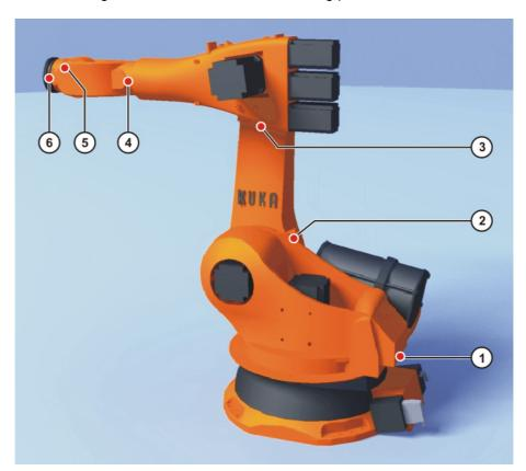
Fig. 5-4: Mastering marks on the robot
