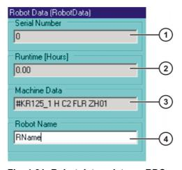
Fig. 4-31: Robot data – data on RDC and hard drive are identical
