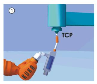
Fig. 5-17: Moving to the external TCP
