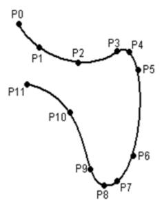
Fig. 8-14: Curved path with spline block
