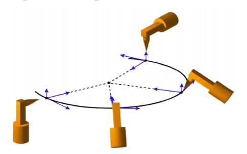
Fig. 8-10: Variable orientation, path-related **\$ORI\_TYPE = #CONSTANT, \$CIRC\_TYPE = #BASE:**
