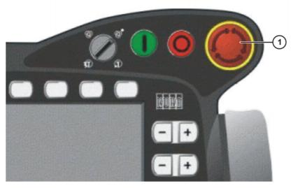
Fig. 3-3: EMERGENCY STOP button on the KCP
