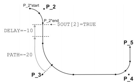
Fig. 10-13: Example of TRIGGER WHEN PATH
