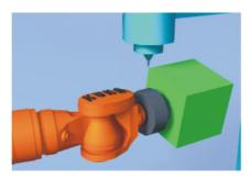
Fig. 5-22: Moving to a known point on the TCP
