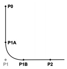
Fig. 8-24: Approximated motion - spline motion
