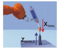
Fig. 5-11: Move to point from 3rd and 4th direction
