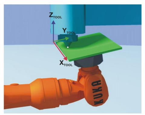
Fig. 5-21: Point on XY plane with a positive Y value
