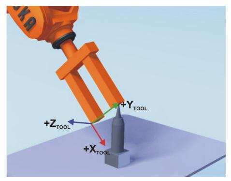
Fig. 5-16: Reference point on XY plane
