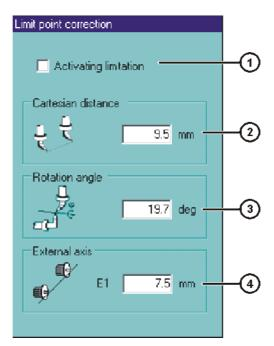
Fig. 6-10: Option window "Limit point correction"
