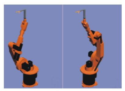
Fig. 8-29: Example: Same TCP position, different axis position
