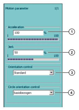
Fig. 9-10: Option window "Motion parameter" (spline motion)
