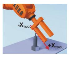
Fig. 5-15: Reference point on the X-axis
