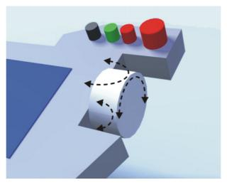
Fig. 4-21: Rotating and tilting the Space Mouse
