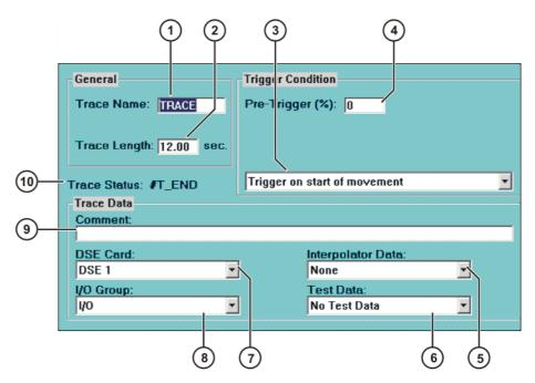
Fig. 12-6: Oscilloscope configuration – main window
