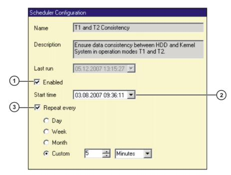
Fig. 6-24: Configuring T1 and T2 Consistency
