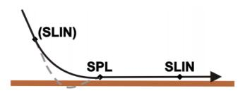
Fig. 9-8: Avoiding a collision with the work surface
