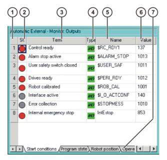
Fig. 4-28: Automatic External outputs (detail view)
