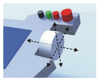
Fig. 4-20: Pushing and pulling the Space Mouse
