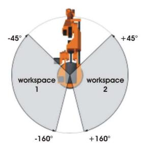
Fig. 6-6: Example of axis-specific workspaces for A1
