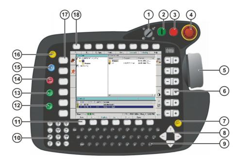
Fig. 4-1: Front view of KCP
