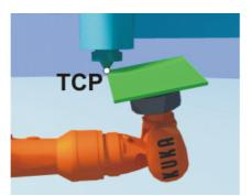
Fig. 5-19: Origin of the workpiece coordinate system
