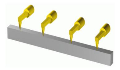
Fig. 8-7: Orientation control - Constant
