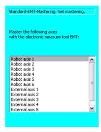
Fig. 5-7: Selection list of axes to be mastered
