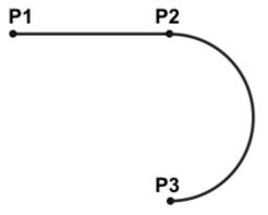
Fig. 8-15: Exact positioning at P2
