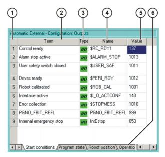
Fig. 6-17: Configuring Automatic External outputs
