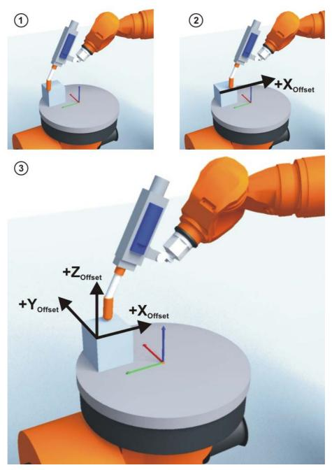
Fig. 5-30: Base calibration principle
