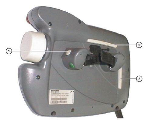
Fig. 3-4: Enabling switches on the KCP
