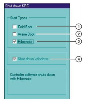
Fig. 4-15: Option window "Shut down KRC"
