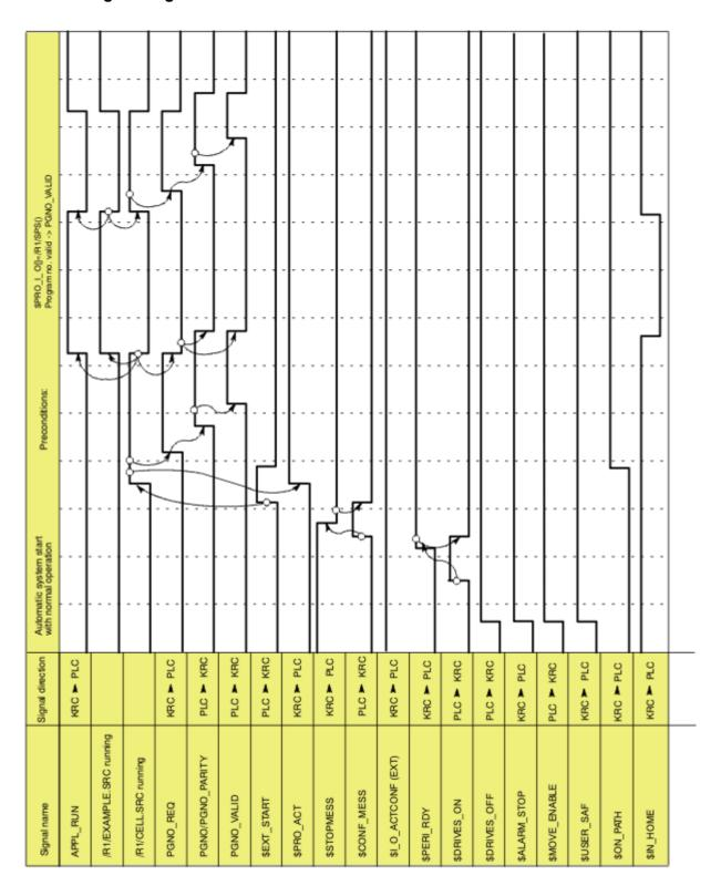
Fig. 6-18: Automatic system start and normal operation with program number acknowledgement by means of PGNO\_VALID
