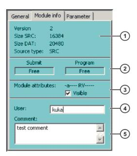
Fig. 7-3: File properties, "Module info" tab
