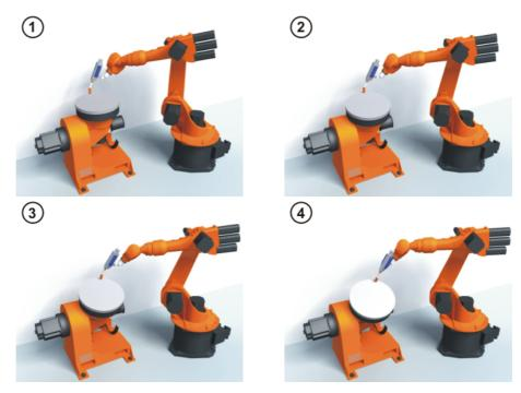
Fig. 5-29: Root point calibration principle
