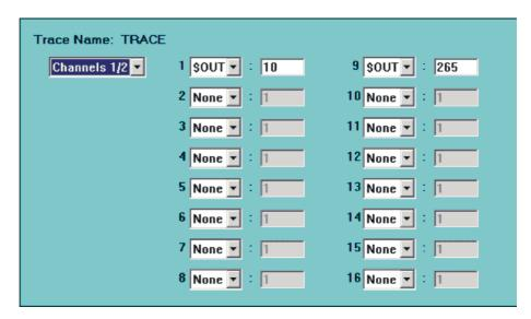
Fig. 12-9: Example: 2 outputs are recorded, 2 channels = 2 colors
