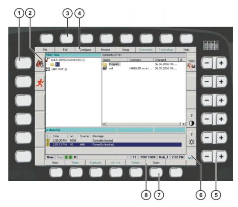
Fig. 4-6: Status keys, menu keys and softkeys in the user interface
