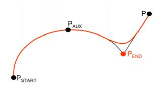
Fig. 8-6: CIRC motion, P<sub>END</sub> is approximated
