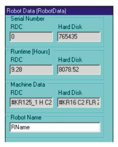
Fig. 4-32: Robot data - data on RDC and hard drive are not identical
