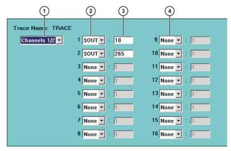
Fig. 12-8: Example: 2 outputs are recorded, 1 channel = 1 color
