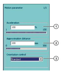
Fig. 9-6: Option window "Motion parameter" (LIN, CIRC)
