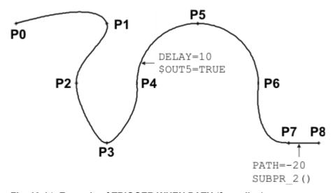
Fig. 10-14: Example of TRIGGER WHEN PATH (for spline)
