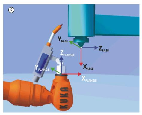
Fig. 5-18: Aligning the coordinate systems parallel to one another
