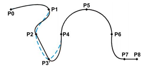
Fig. 8-21: Segment type has been changed
