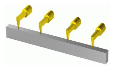
Fig. 8-27: Orientation control - Constant
