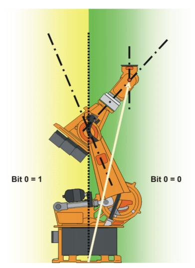
Fig. 8-30: Example: The intersection of the wrist axes (red dot) is in the basic area.
