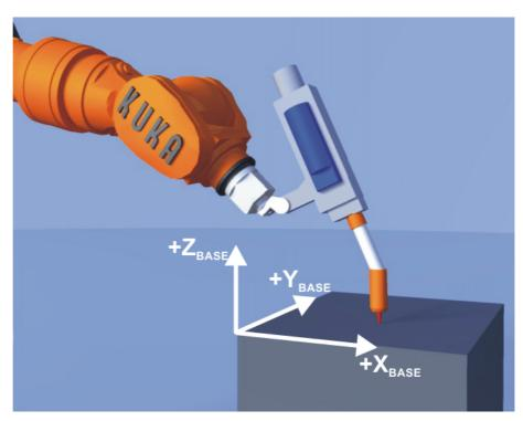
Fig. 5-26: Point on XY plane with a positive Y value
