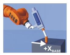
Fig. 5-25: Point on the positive X axis
