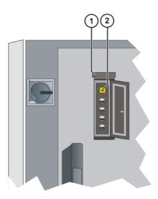
Fig. 4-5: KCP coupler LEDs and request button
