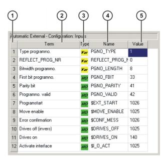
Fig. 6-16: Configuring Automatic External inputs
