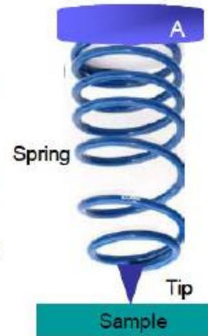
Figure 1. a) Spring depiction of cantilever b) SEM image of triangular SPM cantilever with probe (tip). (Image from MikroMasch ) 1
