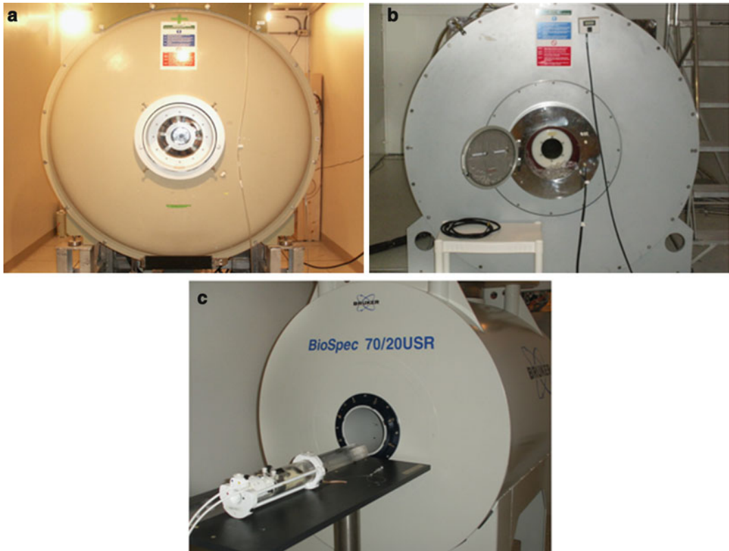
Fig. 1. Small animal MRI scanners available from various companies. (a) shows a refurbished 200 MHz 40 cm bore Oxford NMR system with passive shielding inside a Faraday cage. The scanner is lower in cost than actively shielded and new systems, but can be used for a variety of applications in rodents and small primates. (b) shows a 200 MHz 40 cm bore system from Magnex Scientific of similar dimensions. This system is actively shielded and contains a shielded front and back panel door to reduce MR field fluctuations. Both systems in (a) and (b) are filled with cryogens on a weekly basis. (c) shows an actively shielded 300 MHz Bruker USA 20 cm bore system with cryogen recapture system and coldhead for zero helium boil-off. This system also has a bed (not shown) that is used to move the RF coil along with the animal to adjust positioning inside the system.
