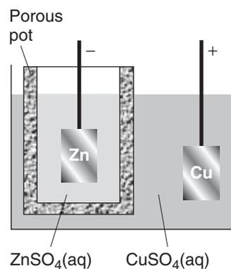
**Fig. 5.9** A Daniell cell consists of copper in contact with copper(II) sulfate solution and zinc in contact with zinc sulfate solution; the two compartments are in contact through the porous pot that contains the zinc sulfate solution. The copper electrode is the cathode and the zinc electrode is the anode.
