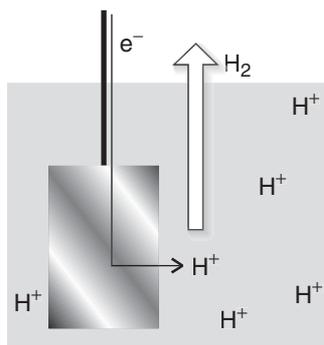
**Fig. 5.7** The schematic structure of a hydrogen electrode, which is like other gas electrodes. Hydrogen is bubbled over a black (that is, finely divided) platinum surface that is in contact with a solution containing hydrogen ions. The platinum, as well as acting as a source or sink for electrons, speeds the electrode reaction because hydrogen attaches to (adsorbs on) the surface as atoms.
