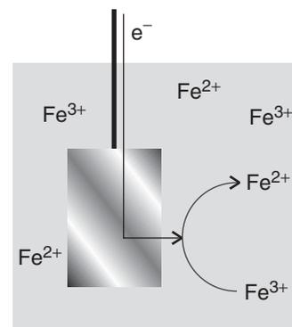
**Fig. 5.8** The schematic structure of a redox electrode. The platinum metal acts as a source or sink for electrons required for the interconversion of (in this case)  $\text{Fe}^{2+}$  and  $\text{Fe}^{3+}$  ions in the surrounding solution.
