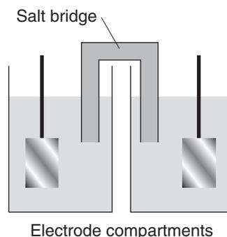
**Fig. 5.4** When the electrolytes in the electrode compartments of a cell are different, they need to be joined so that ions can travel from one compartment to another. One device for joining the two compartments is a salt bridge.
