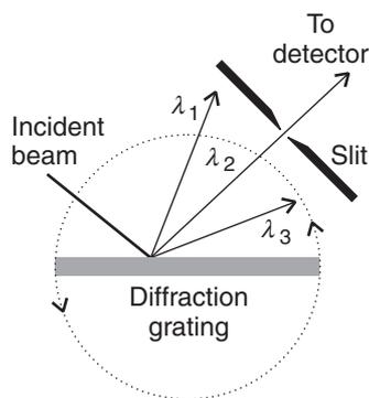
**Fig. 13.4** A beam of light is dispersed by a diffraction grating into three component wavelengths  $\lambda_1$ ,  $\lambda_2$ , and  $\lambda_3$ . In the configuration shown, only radiation with  $\lambda_2$  passes through a narrow slit and reaches the detector. Rotating the diffraction grating in the direction shown by the double arrows allows other wavelengths to reach the detector.
