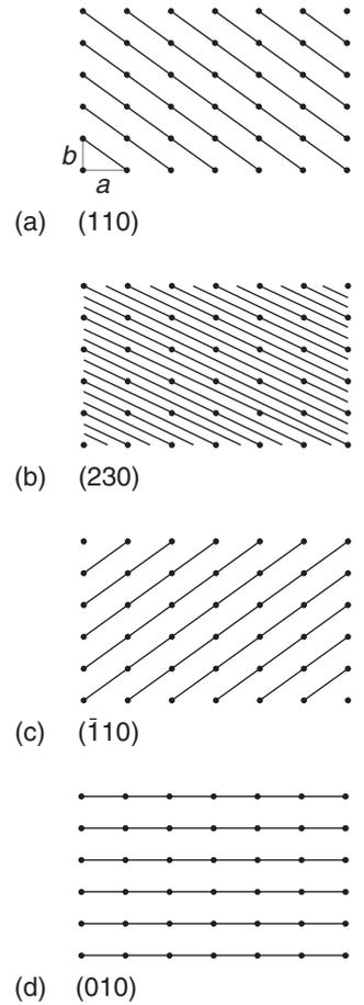
**Fig. 11.9** Some of the planes that can be drawn through the points of the space lattice and their corresponding Miller indices  $(hkl)$ .
