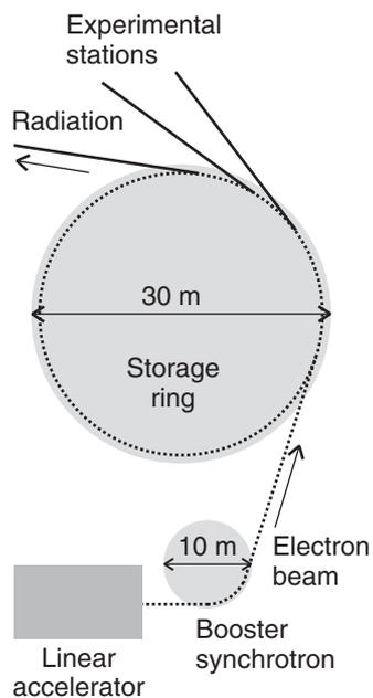
**Fig. 11.23** A synchrotron storage ring. The electrons injected into the ring from the linear accelerator and booster synchrotron are accelerated to high speeds in the main ring. An electron in a curved path is subject to constant acceleration, and an accelerated charge radiates electromagnetic energy.
