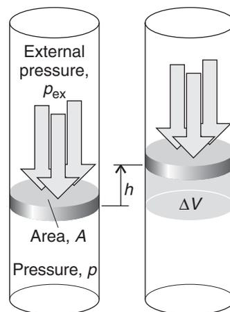
**Fig. 1.9** When a piston of area  $A$  moves out through a distance  $h$ , it sweeps out a volume  $\Delta V = Ah$ . The external pressure  $p_{\text{ex}}$  opposes the expansion with a force  $p_{\text{ex}}A$ .
