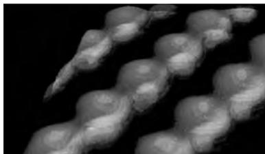
**Fig. 9.23** An STM image of cesium atoms on a gallium arsenide surface.
