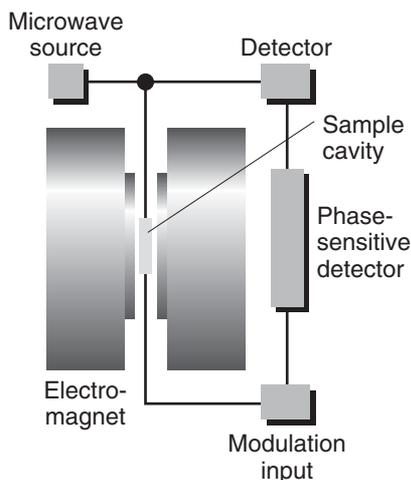
**Fig. 14.42** The layout of a continuous-wave EPR spectrometer. A typical magnetic field is 0.3 T, which requires microwaves of frequency 9 GHz (wavelength 3 cm) for resonance.
