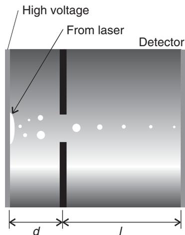
**Fig. 11.2** Diagram of a matrix-assisted laser desorption/ionization time-of-flight (MALDI-TOF) mass spectrometer. A laser beam ejects macromolecules and ions from the solid matrix. The ionized macromolecules are accelerated by an electrical potential difference over a distance  $d$  and then travel through a drift region of length  $l$ . Ions with the smallest mass to charge ratio ( $m/z$ ) reach the detector first.
