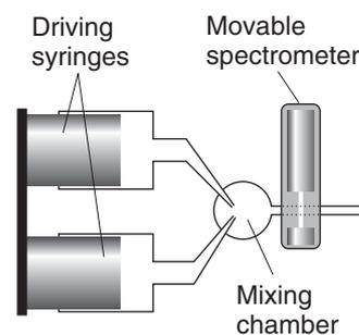
**Fig. 6.3** The arrangement used in the flow technique for studying reaction rates. The reactants are squirted into the mixing chamber at a steady rate from the syringes or by using peristaltic pumps (pumps that squeeze the fluid through flexible tubes, like in our intestines). The location of the spectrometer corresponds to different times after initiation.
