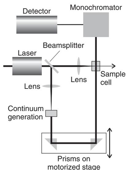
**Fig. 13.48** A configuration used for time-resolved absorption spectroscopy, in which the same pulsed laser is used to generate a monochromatic pump pulse and, after continuum generation in a suitable liquid, a “white” light probe pulse. The time delay between the pump and probe pulses may be varied.
