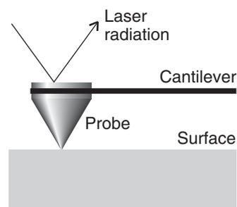
**Fig. 9.25** In atomic force microscopy, a laser beam is used to monitor the tiny changes in position of a probe as it is attracted to or repelled by atoms on a surface.
