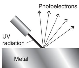
**Fig. 9.3** The experimental arrangement to demonstrate the photoelectric effect. A beam of ultraviolet radiation is used to irradiate a patch of the surface of a metal, and electrons are ejected from the surface if the frequency of the radiation is above a threshold value that depends on the metal.
