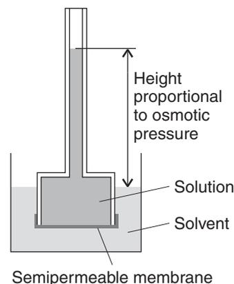
**Fig. 3.33** In a simple osmosis experiment, a solution is separated from the pure solvent by a semipermeable membrane. Pure solvent passes through the membrane and the solution rises in the inner tube. The net flow ceases when the pressure exerted by the column of liquid is equal to the osmotic pressure of the solution.
