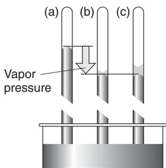
**Fig. 3.6** When a small volume of water is introduced into the vacuum above the mercury in a barometer (a), the mercury is depressed (b) by an amount that is proportional to the vapor pressure of the liquid. (c) The same pressure is observed however much liquid is present (provided some is present).
