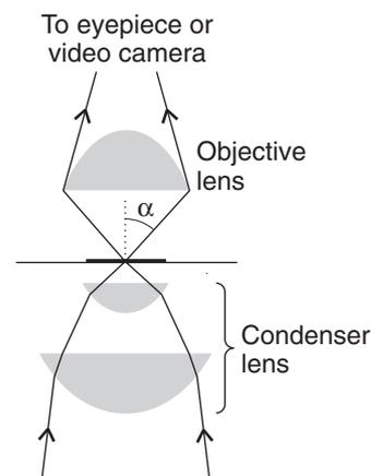
**Fig. 13.25** The light path in a typical microscope, with rays shown in gray and their directions shown by arrowheads. Light is focused by the condenser lens (typically a system of two lenses), scattered by the sample, and refocused by an objective lens. The ability of the objective lens to resolve two objects into distinct images depends on the numerical aperture, which is related to the refractive index of the lens material and the angle  $\alpha$ , as discussed in the text.
