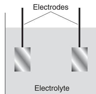
**Fig. 5.3** The arrangement for an electrochemical cell in which the two electrodes share a common electrolyte.
