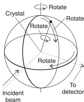
**Fig. 11.21** The geometry of a four-circle diffractometer. The settings of the orientations of the components is controlled by computer; each reflection is monitored in turn, and their intensities are recorded.
