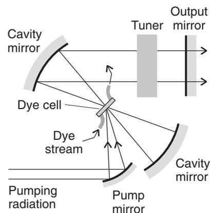
**Fig. 13.59** The configuration used for a dye laser. The dye is flowed through the cell inside the laser cavity. The flow helps to keep it cool and prevents degradation.
