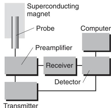
**Fig. 14.3** The layout of a typical NMR spectrometer. The link from the transmitter to the detector indicates that the high frequency of the transmitter is subtracted from the high-frequency received signal to give a low-frequency signal for processing.
