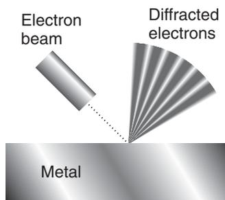
**Fig. 9.5** In the Davisson-Germer experiment, a beam of electrons was directed on a single crystal of nickel, and the scattered electrons showed a variation in intensity with angle that corresponded to the pattern that would be expected if the electrons had a wave character and were diffracted by the layers of atoms in the solid.
