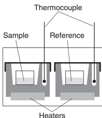
**Fig. 1.21** A differential scanning calorimeter.
