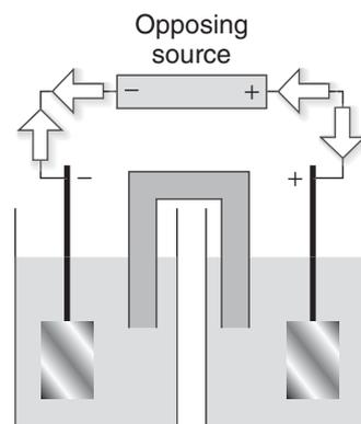
**Fig. 5.10** The emf is measured by balancing the cell against an external potential that opposes the reaction in the cell. When there is no current flow, the external potential difference is equal to the emf of the cell.
