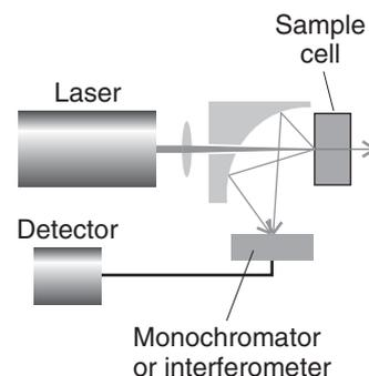
**Fig. 13.5** A common arrangement adopted in Raman spectroscopy. A laser beam first passes through a lens and then through a small hole in a mirror with a curved reflecting surface. The focused beam strikes the sample and scattered light is both deflected and focused by the mirror. The spectrum is analyzed by a monochromator or an interferometer.
