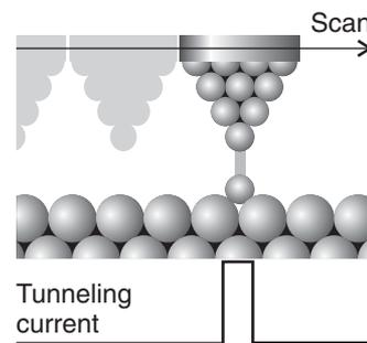
**Fig. 9.22** A scanning tunneling microscope makes use of the current of electrons that tunnel between the surface and the tip. That current is very sensitive to the height of the tip above the surface.
