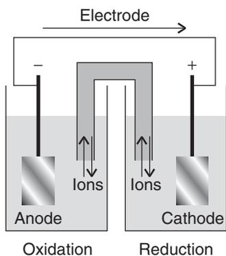
**Fig. 5.5** The flow of electrons in the external circuit is from the anode of a galvanic cell, where they have been lost in the oxidation reaction, to the cathode, where they are used in the reduction reaction. Electrical neutrality is preserved in the electrolytes by the flow of cations and anions in opposite directions through the salt bridge.
