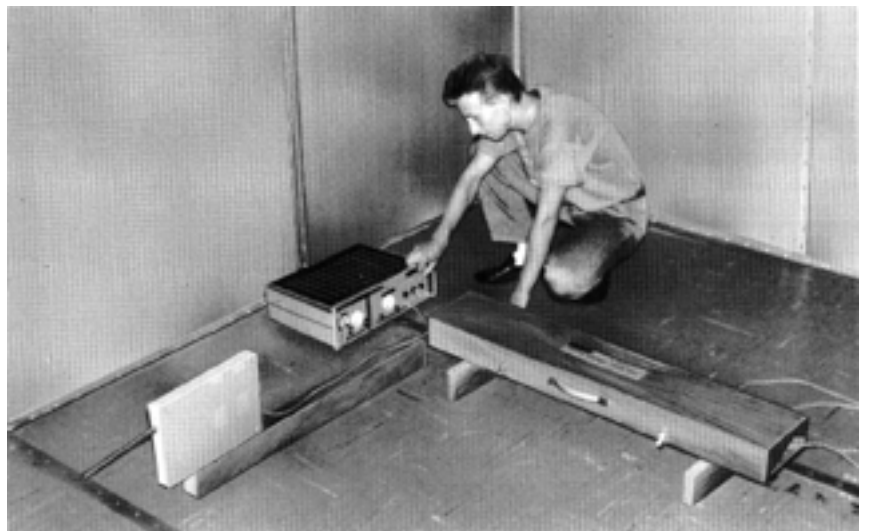
fig. 27: susceptibility to fast transients, measured on an Isis master control unit (test 801-4) in a Faraday room. This photo shows the disturbance generator being adjusted by an operator, the wooden case containing the coupling clamp and the Isis master control unit connected to the Batibus network.
