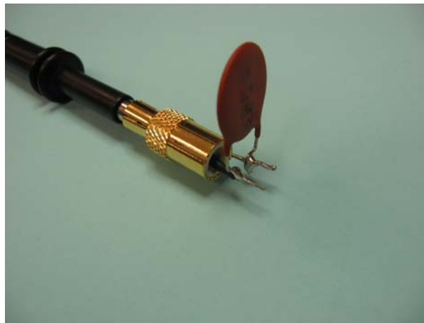
Figure 52 – Oscilloscope Probe with Probe Master ( www.probemaster.com ) 4987A BNC Adapter. Modified with wires for ripple measurement, and one parallel decoupling capacitor added.)
