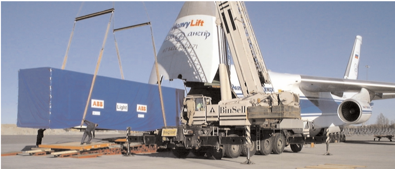
Loading of prefabricated module.
