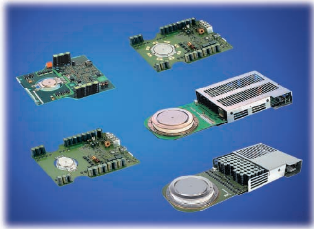
Fig. 3 Standard IGCT sizes
