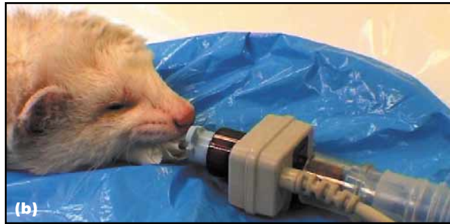
7.8 (a) Close-up of a connector for sampling gas (sidestream capnograph). (b) Adaptor and sensor of a mainstream capnograph.
