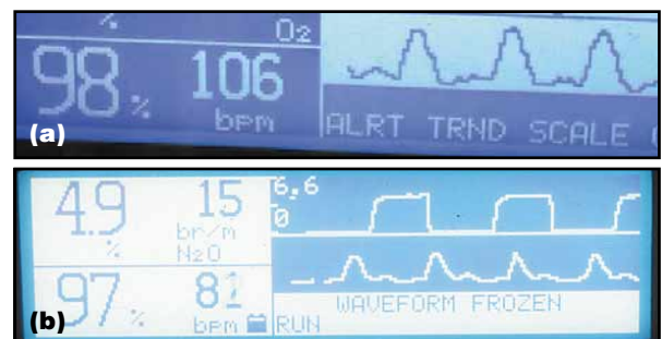
7.18 (a) Pulse oximeter: display of S_pO_2 , heart rate and waveform. (b) Display of capnography and pulse oximetry.
