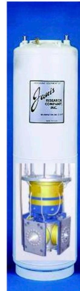
Superconducting magnet  $10 \text{ T}$
