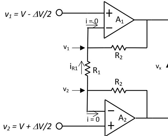
$$i_{R_1} = \frac{(v_2 - v_1)}{R_1}$$
