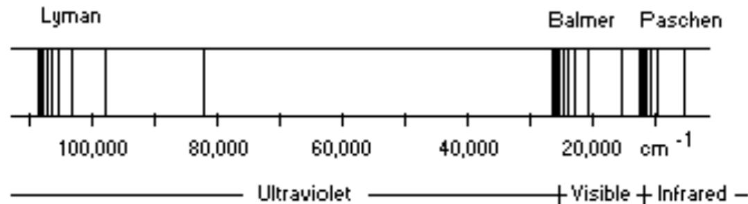
Emission spectrum of heated hydrogen
