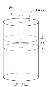
Fig. 2.6 Gas-filled cylinder. There is a constant external pressure,  $p_{ex}$ . For a change in position of the piston,  $\Delta z$ , there is a corresponding change in volume,  $\Delta V$ . The work done by the system is  $w = -p_{ex}\Delta V$ . If  $\Delta V$  is negative, if the gas in the cylinder is compressed, there is a positive contribution to  $\Delta U$ .
