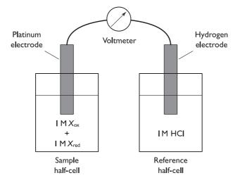
Fig. 4.14 Measurement of the standard redox potential. This device can be used to measure the standard redox potential of a compound. The hydrogen electrode in the reference cell contains I atm H<sub>2</sub>(g).
