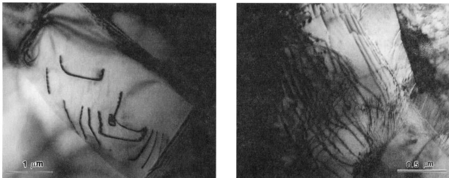
Fig. 4.3: Discordâncias em (a) \text{Al}_2\text{O}_3 and (b) \text{TiC} . (
