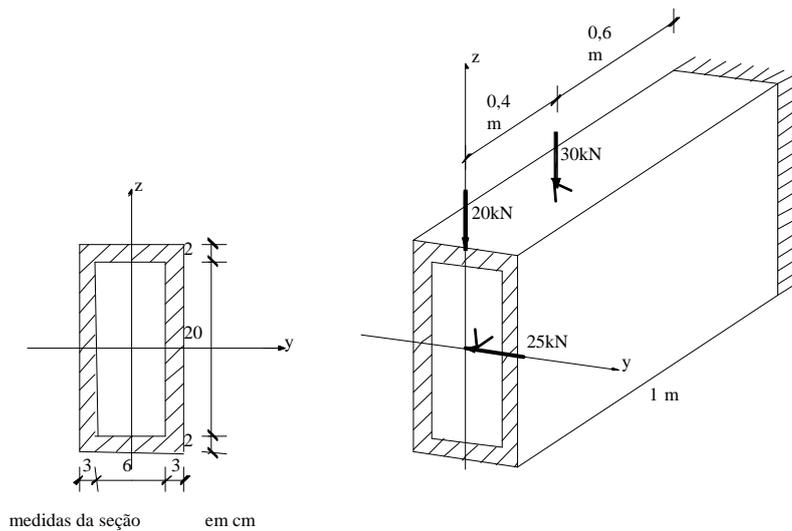
6. Para a viga da figura, com  $P = 35 \text{ kN}$  e  $\sigma_{\text{et}} = \sigma_{\text{ec}} = 25 \text{ kN/cm}^2$ , determine:
