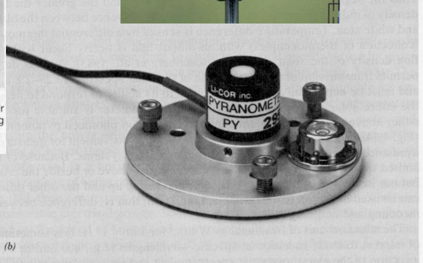
Figure 4.14. Instruments for measuring direct and diffuse solar radiation. (a) Eppley pyranometer (from Sutton et al., 1984; used with permission). (b) Silicon photocell pyranometer (courtesy LI-COR, Inc., Lincoln, NE).
