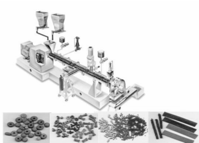
Figure 14.27: Example of a line for cooking-extrusion of dry pet and fish food
