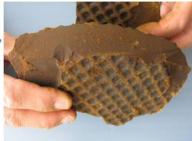
Intermediate lignin filter cake from filtration stage 1
