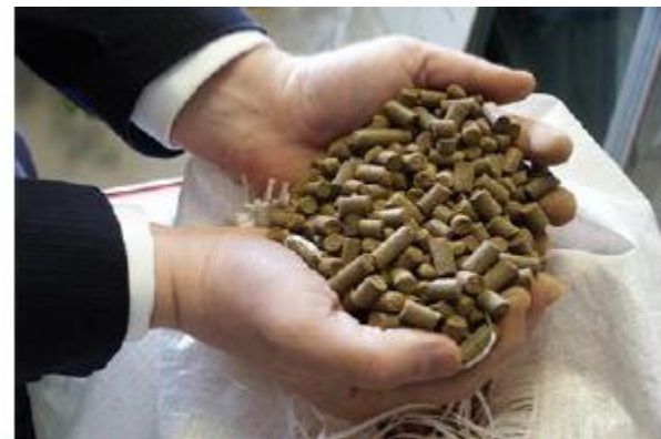
Figure 6. Lignin produced in the demonstration plant at Bäckhammar – filter cake and lignin pellets.
