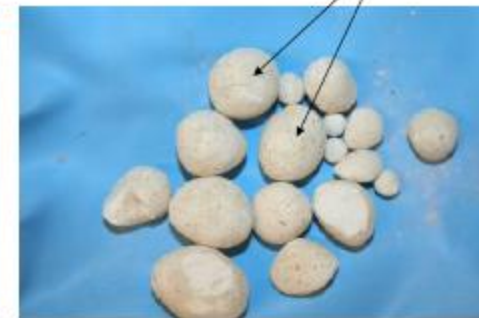
Lime at 100% lignin firing (Sample K32)
