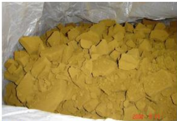
Figure 6. Lignin produced in the demonstration plant at Bäckhammar – filter cake and lignin pellets.
