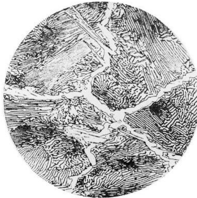
Pearlite and G.B. Cementite in an hypereutectoid steel cementite appears white
