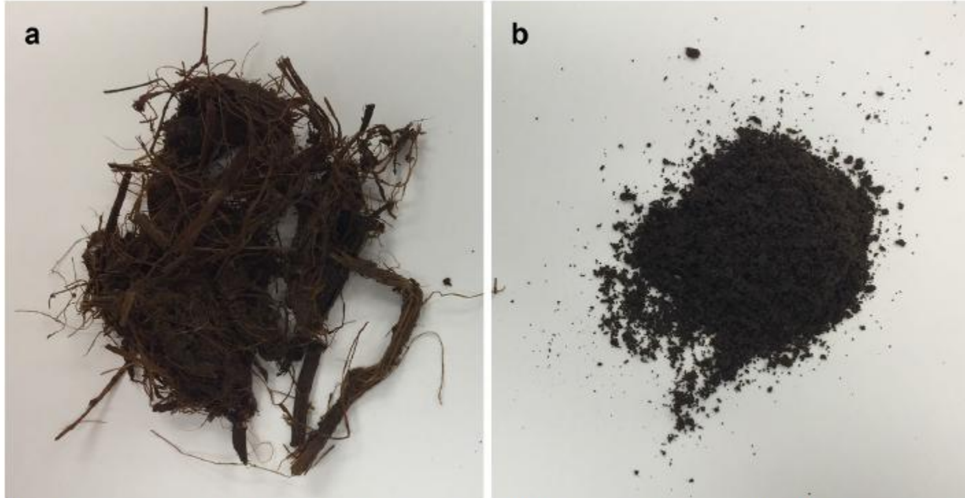
Fig. 6 Size reduction of dilute acid-pretreated corn stover by disk milling. a Dilute acid-pretreated sample; b dilute acid-pretreated and disk-milled sample
