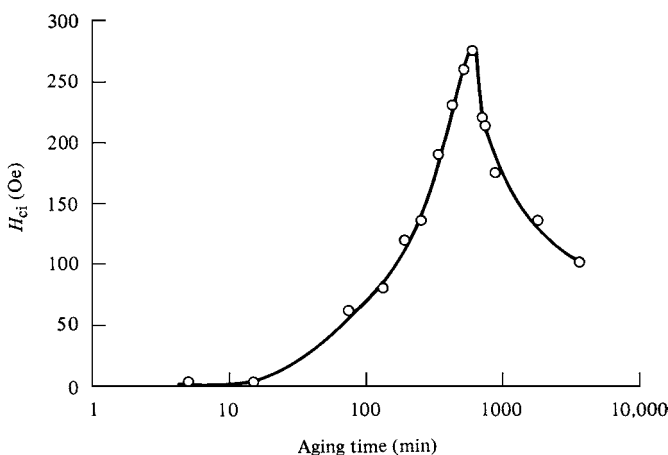
Fig. 11.24 Effect of aging at 700°C on the coercivity H_{ci} of a Cu–Co alloy. [J. J. Becker, Trans. AIME , 209 (1957) p. 59.]
