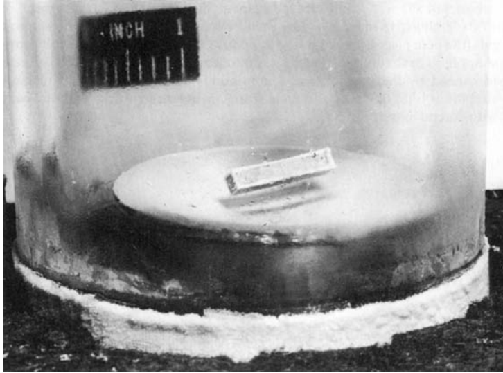
Fig. 14.22 Bar magnet suspended over a superconducting plate.
