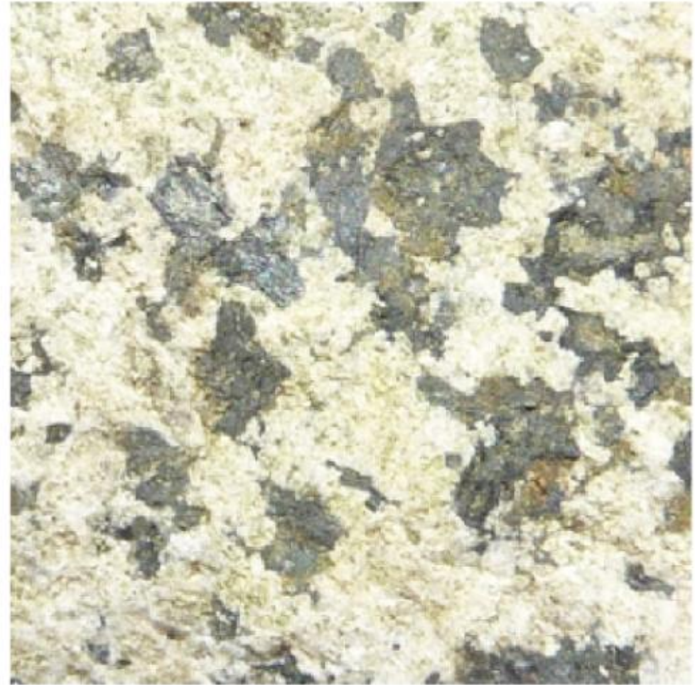
Figure 5.2.1 Unweathered (left) and weathered (right) surfaces of the same piece of granitic rock. On the unweathered surfaces the feldspars are still fresh and glassy-looking. On the weathered surface much of the feldspar has been altered to the chalky-looking clay mineral kaolinite.
