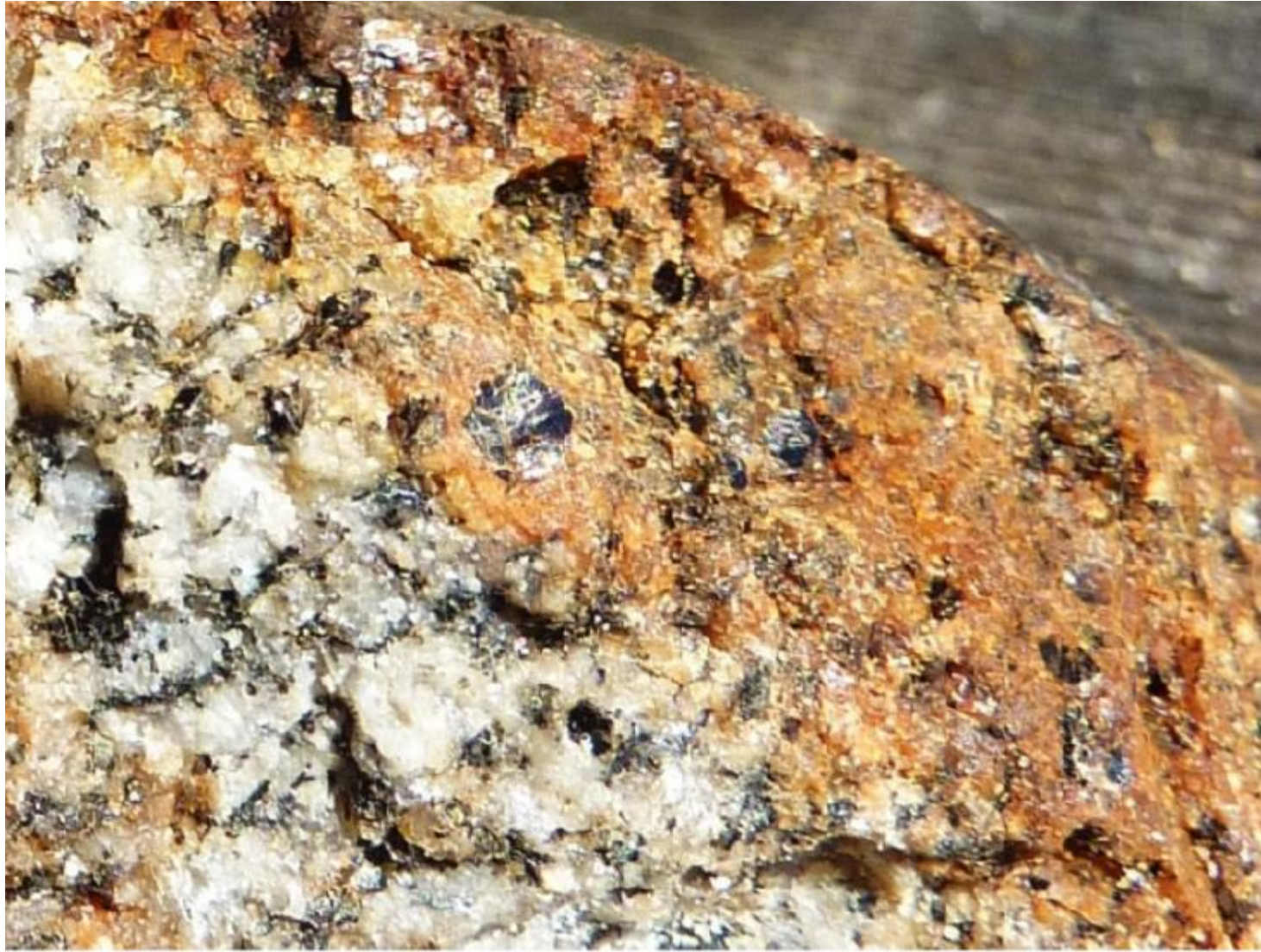
Figure 5.2.2 A granitic rock containing biotite and amphibole which have been altered near to the rock's surface to limonite, which is a mixture of iron oxide minerals.
