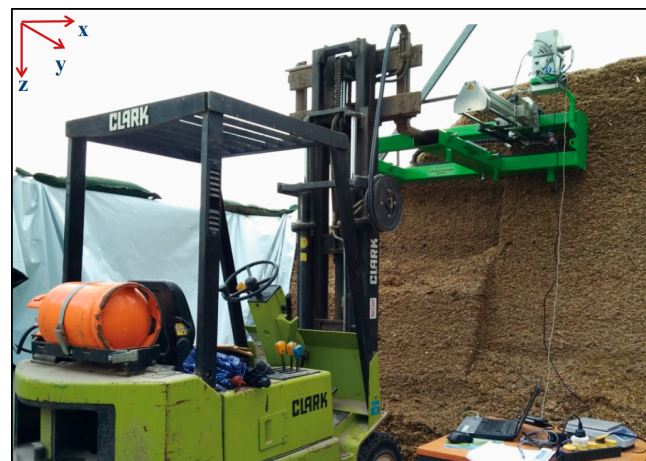
Figure 3. Using a forklift to position the frame prior to penetrating the face of the bunker silo at different heights.
