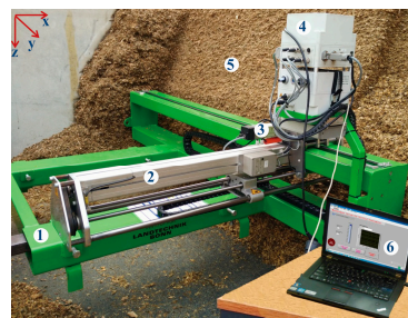
Figure 1. A photo of the penetrometer-based mapping system: (1) frame, (2) penetrometer, (3) motor for y-axis translation, (4) relay-box, (5) maize silo, and (6) the interface of the measurement system.
