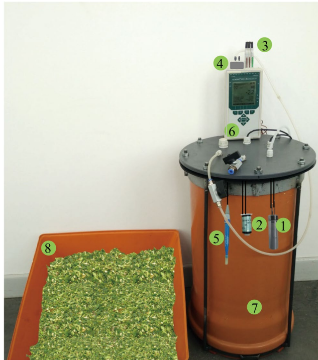
Figure 1. The experimental test silo for both Test-A and Test-B, which included ① CO 2 sensor ② O 2 sensor ③ temperature sensor ④ pH sensor, ⑤ ALMEMO data-logger ⑥ air-tight cylinder and ⑦ test substrate (here fresh chopped maize).
