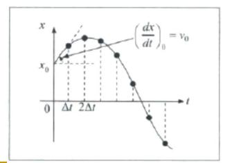
$$\ddot{x} = \frac{d^2x}{dt^2} = -\omega^2 x \qquad \omega = \sqrt{\frac{k}{m}}$$
