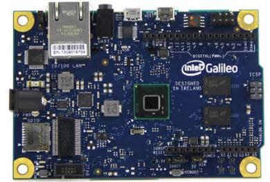
**Intel Quark** *System-on-Chip* (SoC) x1000
