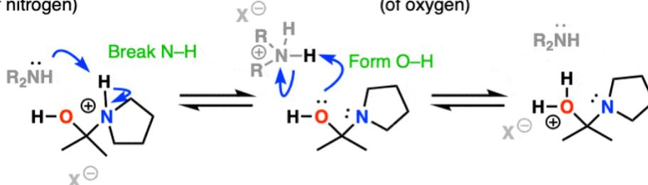
Together, steps 3 and 4 are generically called "proton transfer". The specific identity of the base (in step 3) and acid (in step 4) is generally not crucial, so it's OK to write B and B-H.
