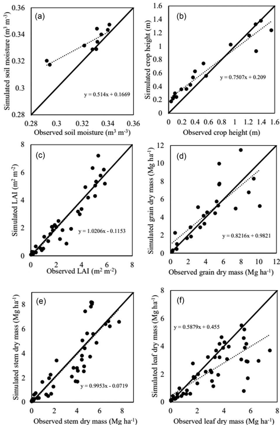
**FIGURE 5** Relationship between simulated and observed values for (a) soil moisture, (b) crop height, (c) leaf area index (LAI), (d) grain dry mass, (e) stem dry mass, (f) leaf dry mass of maize for different regions of Brazil
