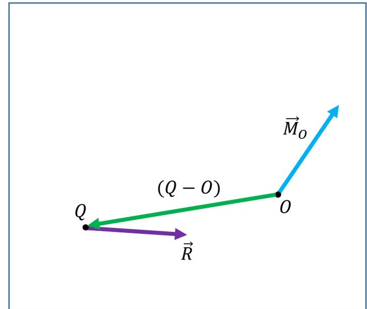
$$\vec{M}_O = \sum_{i=1}^N (P_i - O) \wedge \vec{F}_i = \sum_{i=1}^N (Q - O) \wedge \vec{F}_i = (Q - O) \wedge \sum_{i=1}^N \vec{F}_i \Rightarrow \boxed{\vec{M}_O = (Q - O) \wedge \vec{R}}$$
