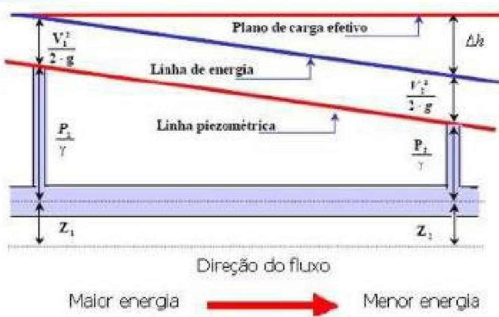
$$z_1 + \frac{P_1}{\gamma} + \frac{V_1^2}{2g} = z_2 + \frac{P_2}{\gamma} + \frac{V_2^2}{2g} + \Delta H_{1-2}$$
